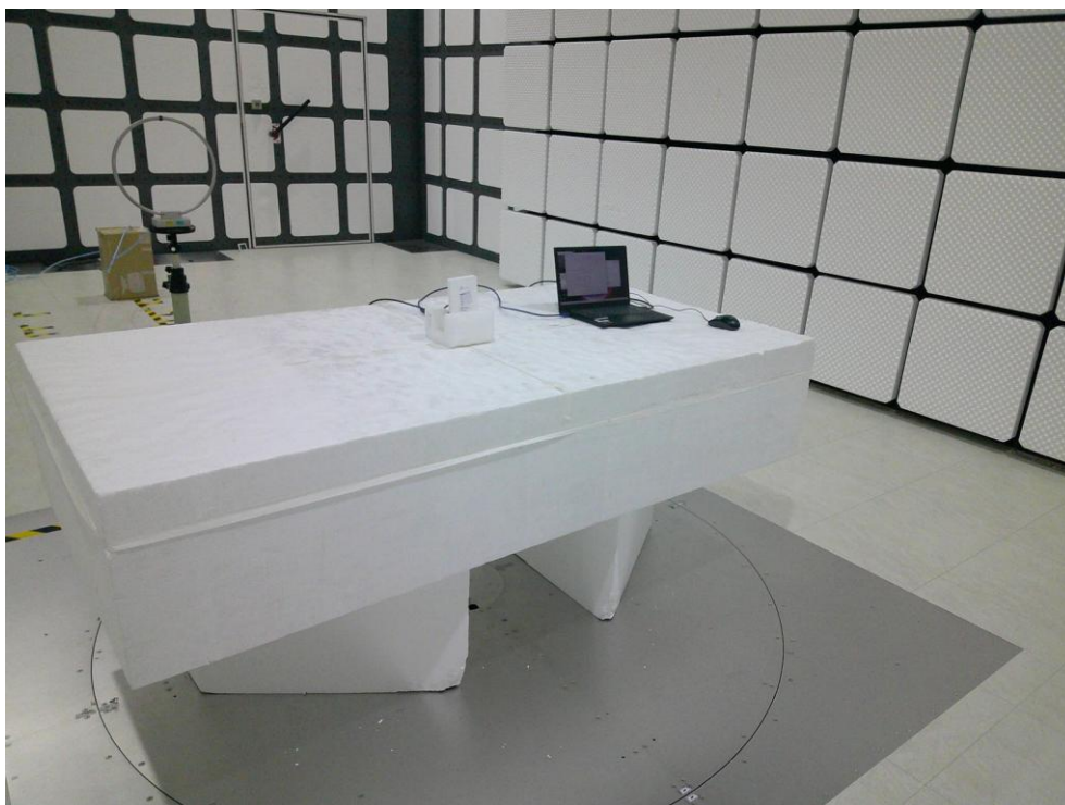
Description: Radiated Emission Test Setup for 9kHz~30MHz
