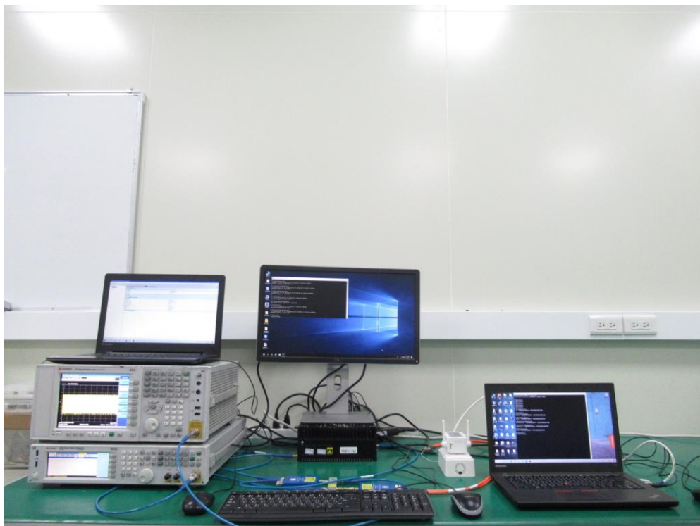
Description: DFS Test Setup
