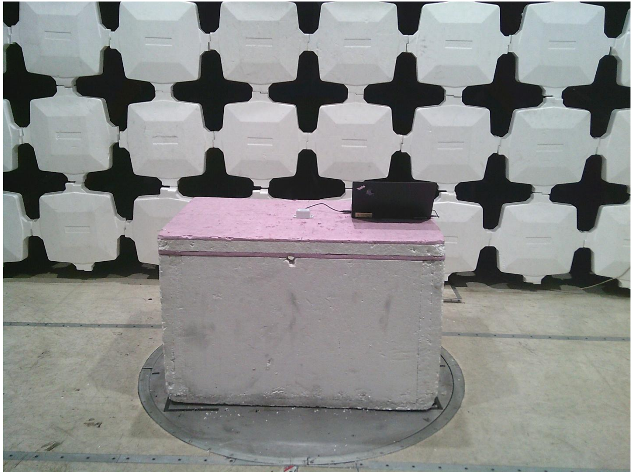
Radiated Testing, Table Setup #1
