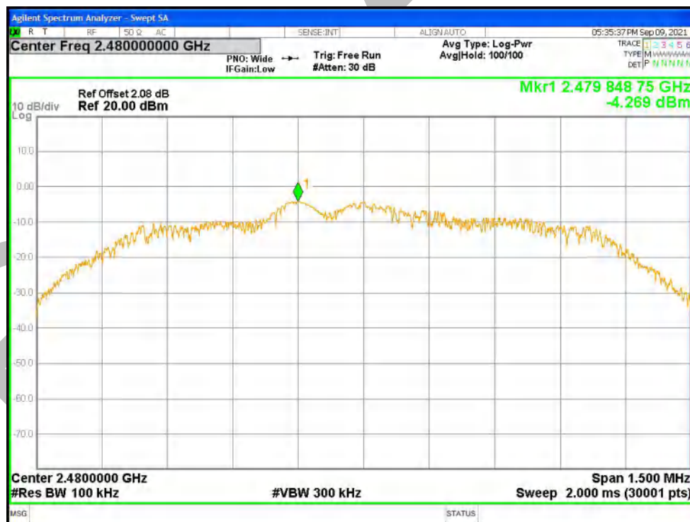
Tx. Spurious NVNT 3-DH1 2480MHz Ant1 Emission
