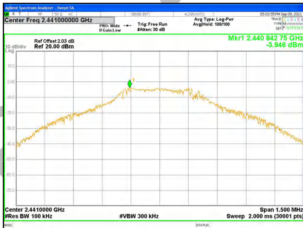
Tx. Spurious NVNT 1-DH1 2441MHz Ant1 Emission
