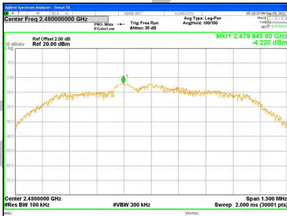
Tx. Spurious NVNT 2-DH1 2480MHz Ant1 Emission
