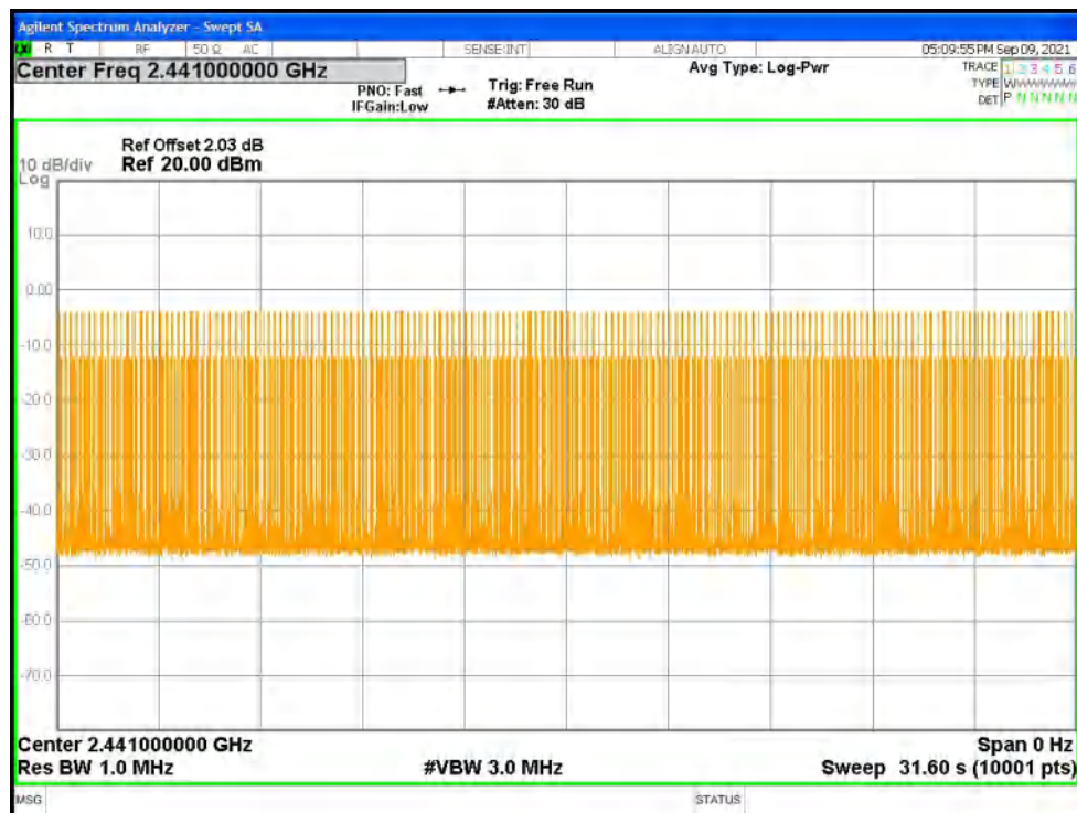
Dwell NVNT 1-DH3 2441MHz Ant1 One Burst
