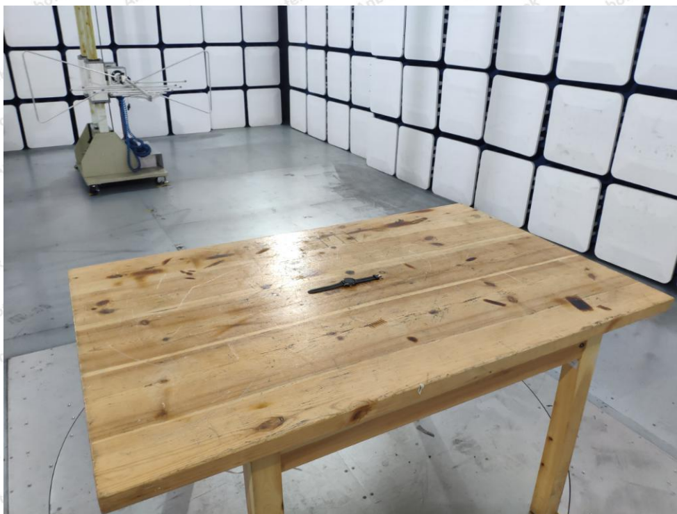
Photo of Radiation Emission Test
