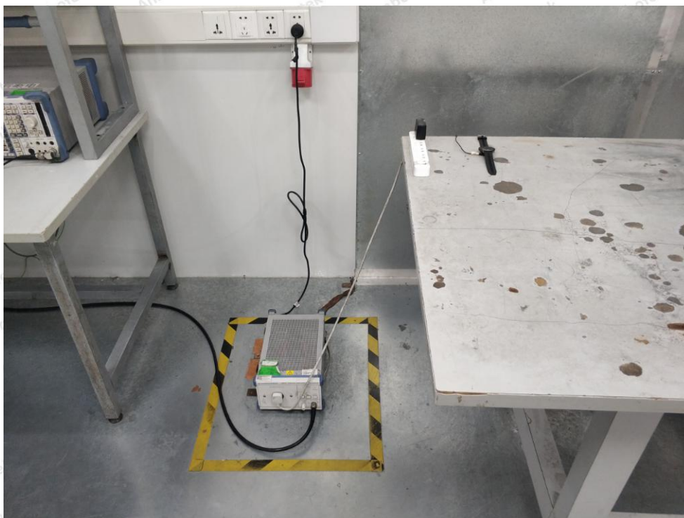
Photo of Conducted Emission Measurement
