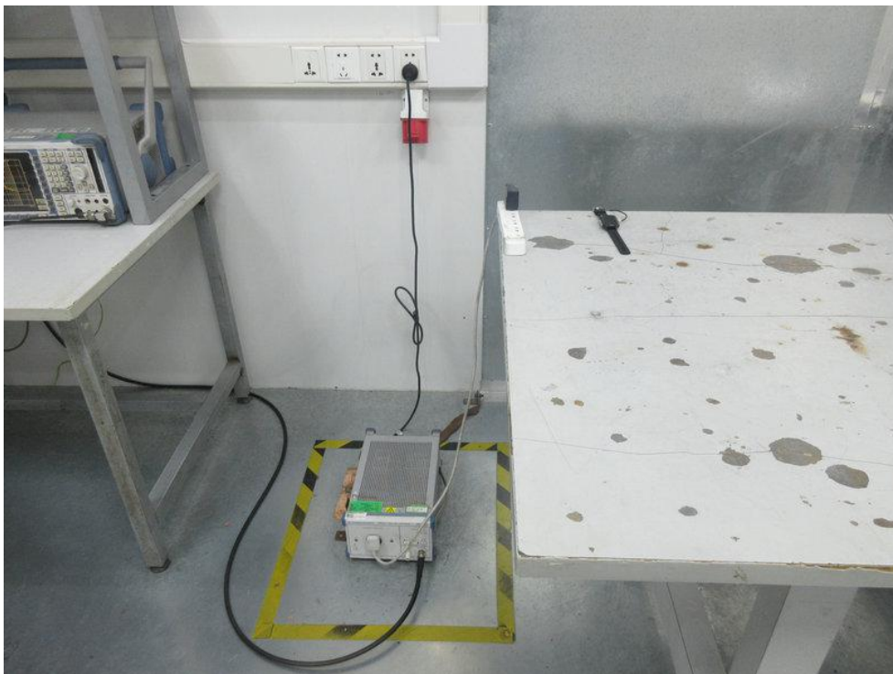
Photo of Conducted Emission Measurement
