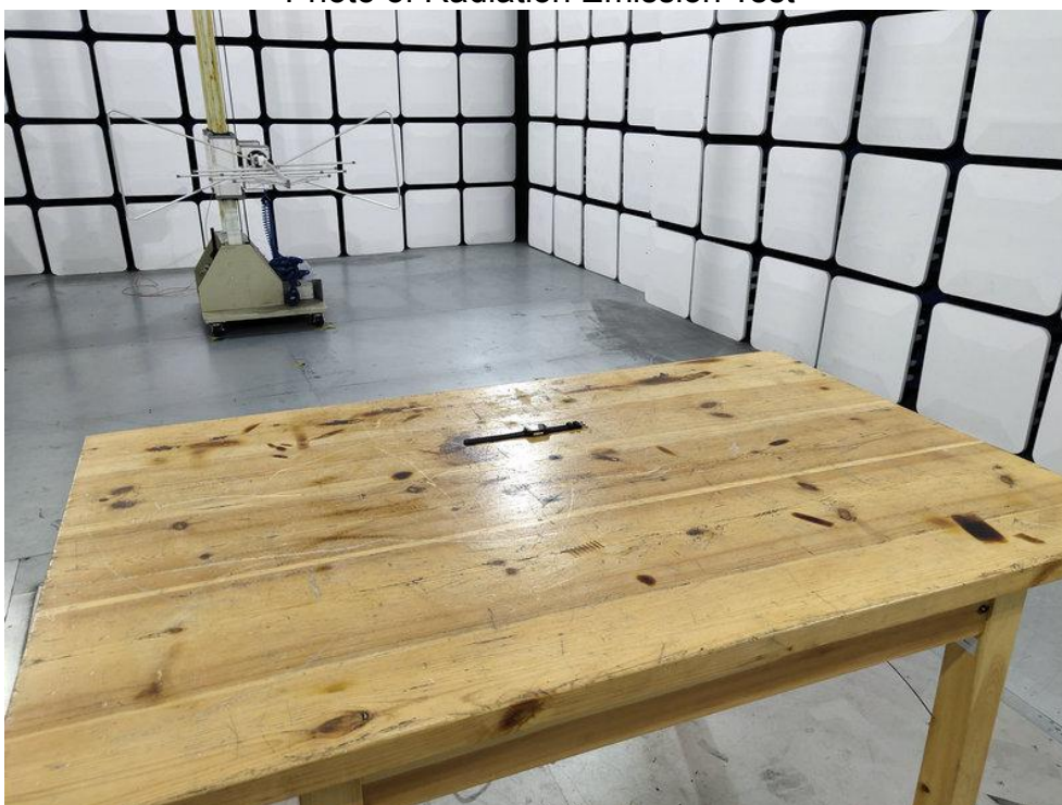
Photo of Radiation Emission Test
