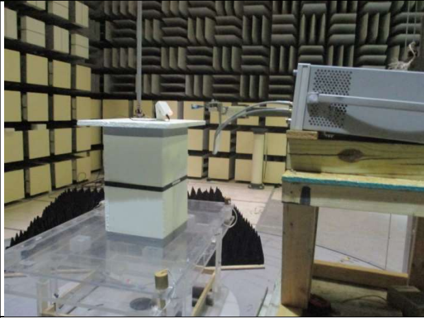
RE Test Setup – 26.5GHz – 40GHz
