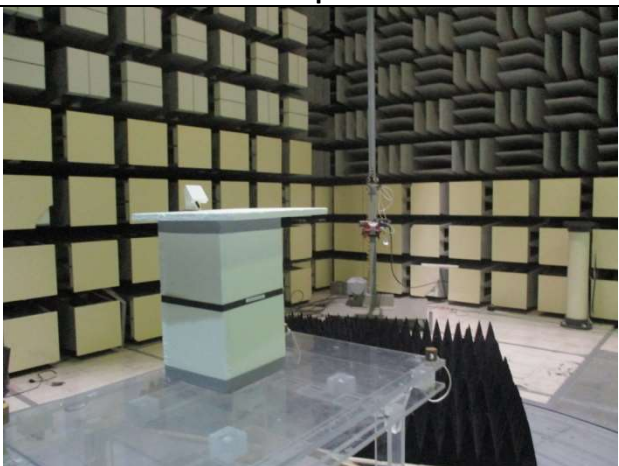
RE Test Setup – 1GHz – 18GHz
