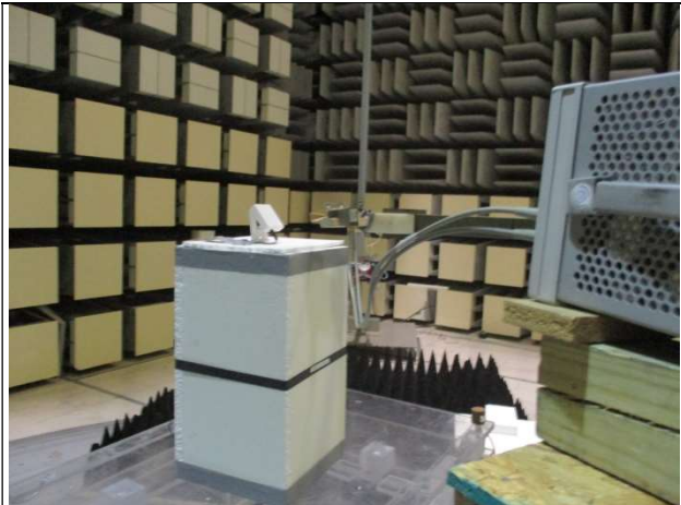
RE Test Setup – 75GHz – 110GHz
