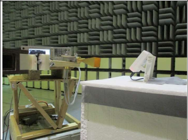
RE Test Setup – 40GHz – 50GHz
