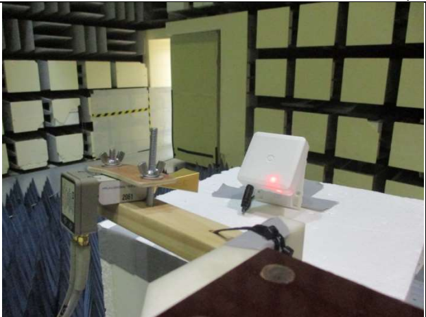
RE Test Setup – 75GHz – 110GHz
