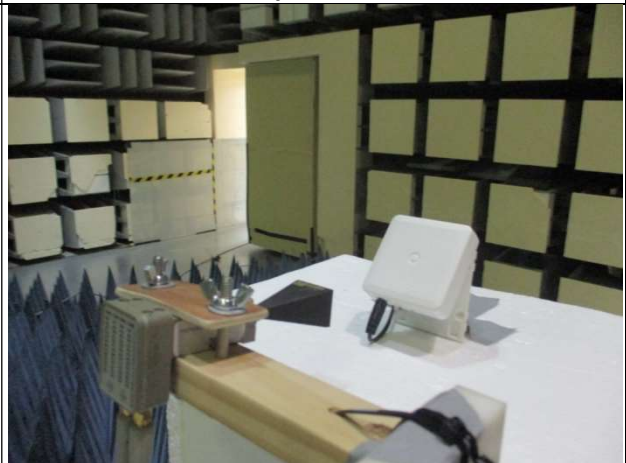
RE Test Setup – 50GHz – 75GHz
