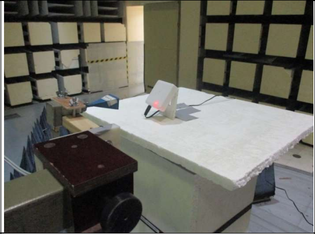
RE Test Setup – 26.5GHz – 40GHz
