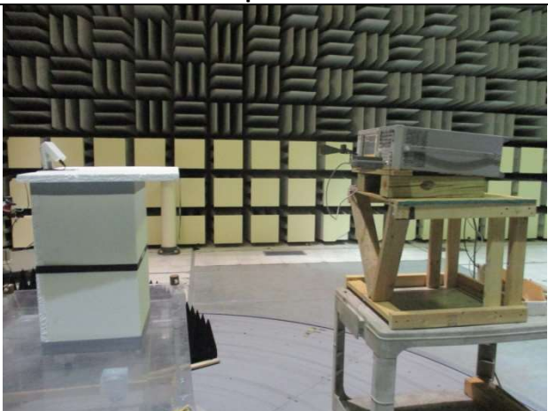
RE Test Setup – 18GHz – 26.5GHz
