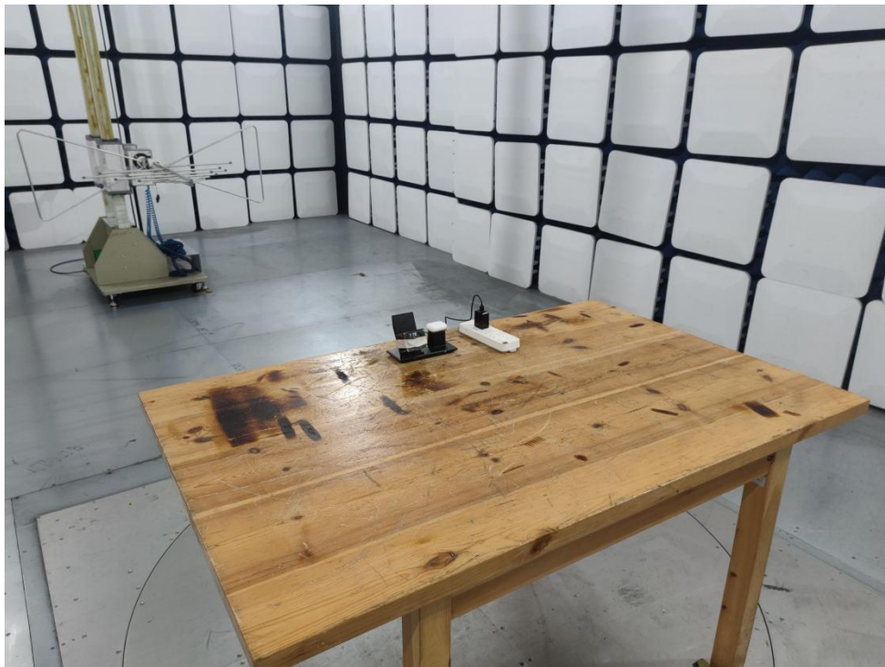
Photo of Radiation Emission Test
