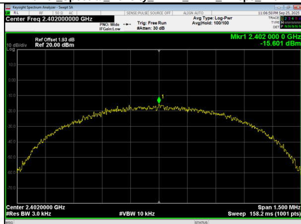
Power Spectral Density NVNT_ANT1_1Mbps_2402
