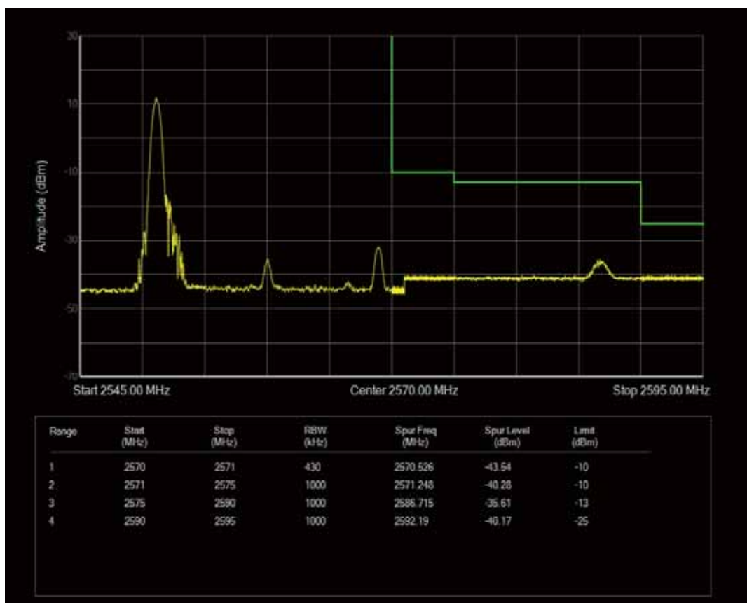
Band7 QAM16 BW=20MHz Channel=21350 RB Size=1 Position=#Max
