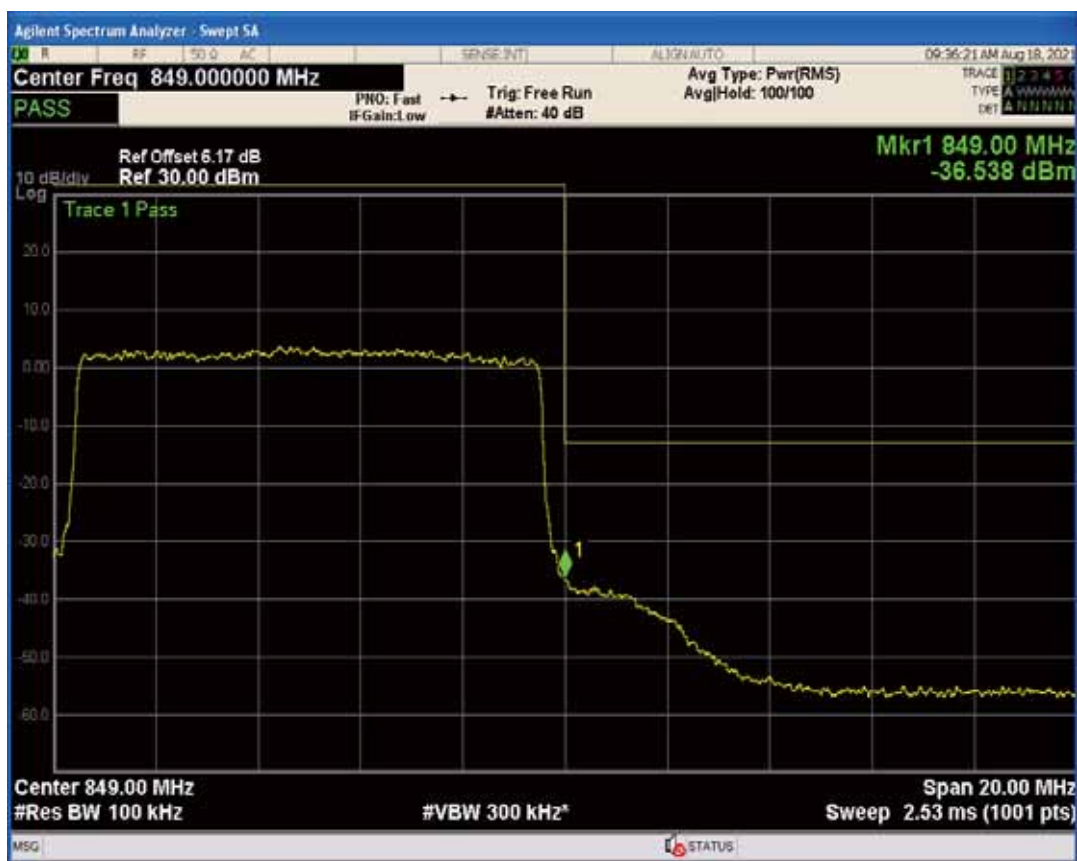
Band5 QPSK BW=10MHz Channel=20600 RB Size=1 Position=#Max
