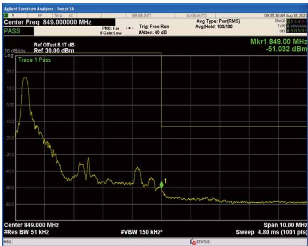
Band5 QAM16 BW=5MHz Channel=20625 RB Size=1 Position=#Max
