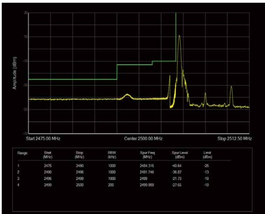
Band7 QAM16 BW=10MHz Channel=20800 RB Size=1 Position=#Max
