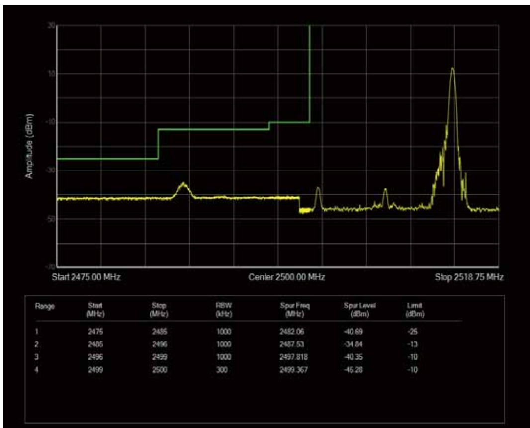
Band7 QPSK BW=15MHz Channel=20825 RB Size=75 Position=#0
