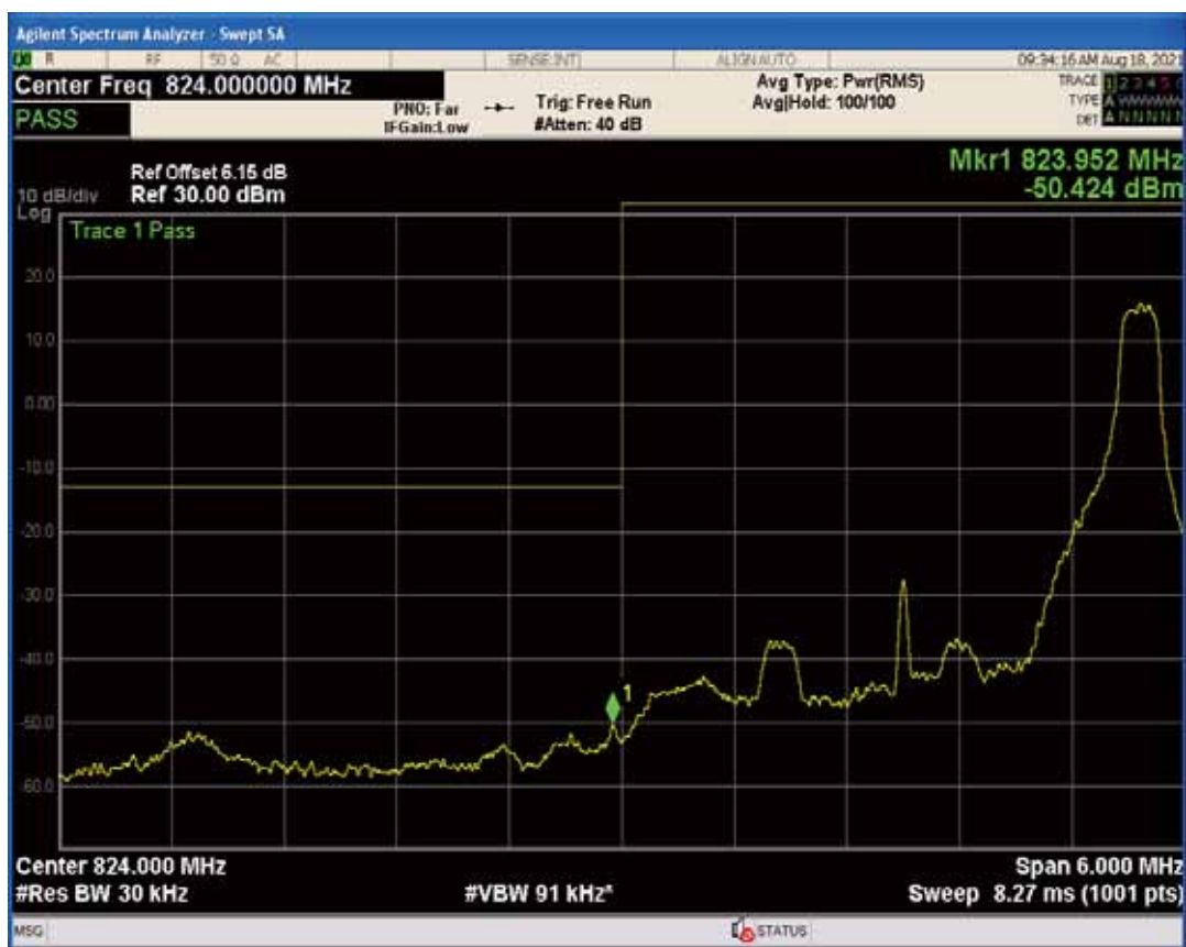
Band5 QPSK BW=3MHz Channel=20415 RB Size=15 Position=#0
