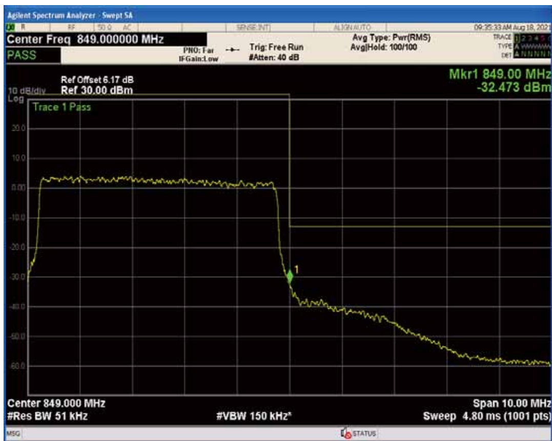
Band5 QAM16 BW=5MHz Channel=20625 RB Size=1 Position=#0
