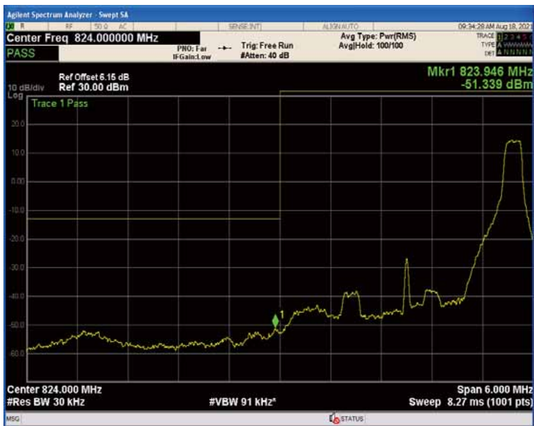
Band5 QAM16 BW=3MHz Channel=20415 RB Size=15 Position=#0
