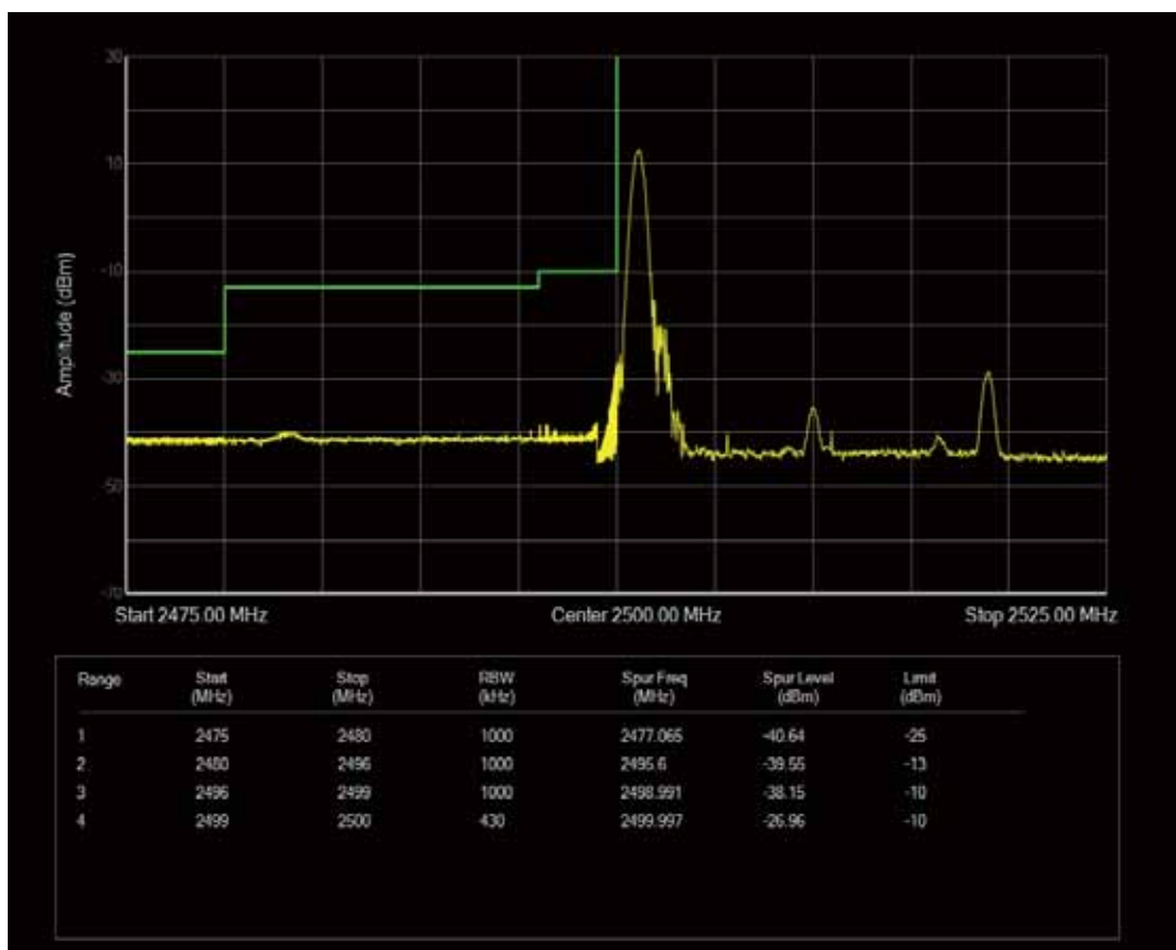
Band7 QPSK BW=20MHz Channel=20850 RB Size=100 Position=#0
