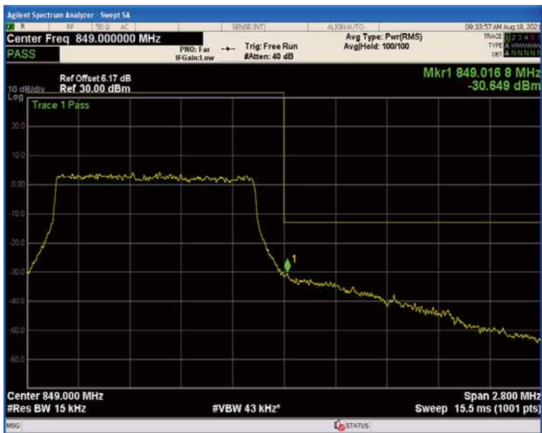
Band5 QAM16 BW=1.4MHz Channel=20643 RB Size=1 Position=#Max
