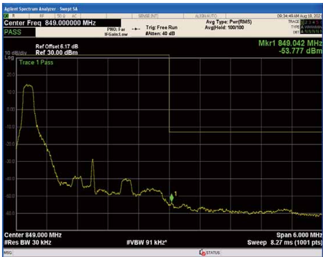
Band5 QPSK BW=5MHz Channel=20425 RB Size=1 Position=#0
