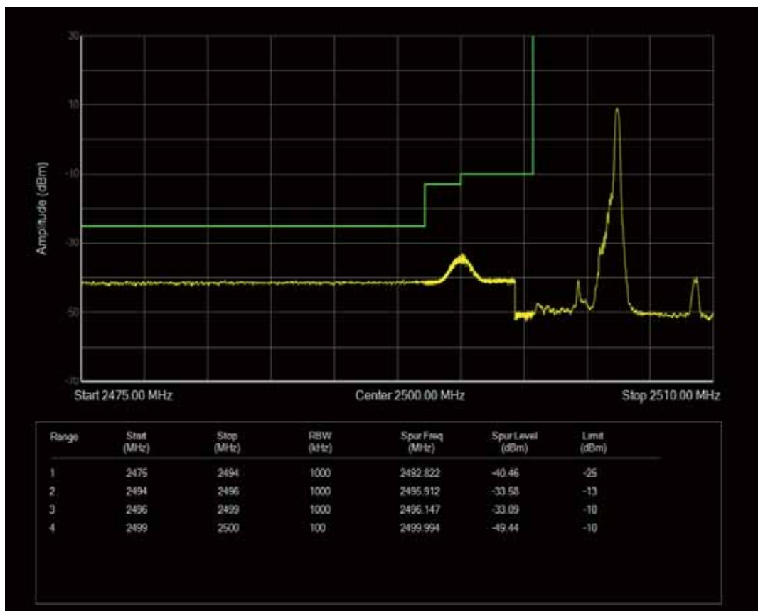
Band7 QAM16 BW=5MHz Channel=20775 RB Size=25 Position=#0
