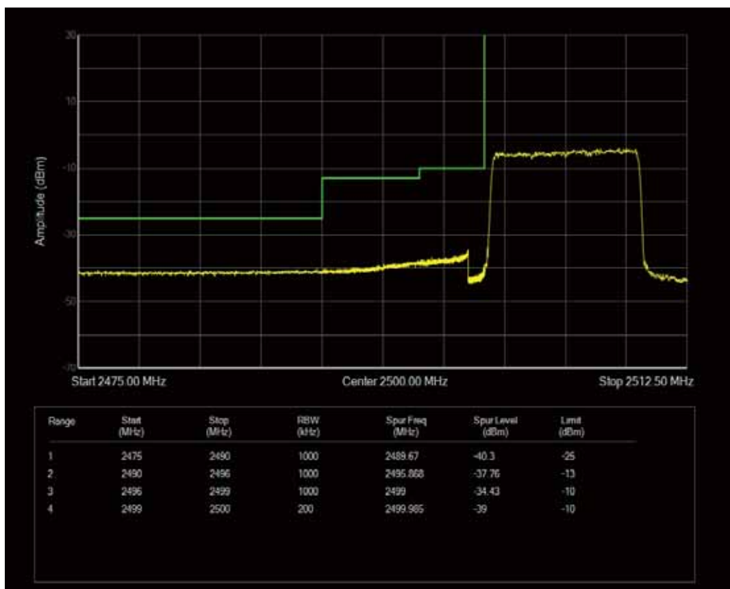
Band7 QPSK BW=10MHz Channel=21400 RB Size=1 Position=#Max
