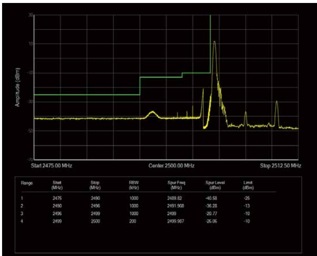
Band7 QPSK BW=10MHz Channel=20800 RB Size=50 Position=#0
