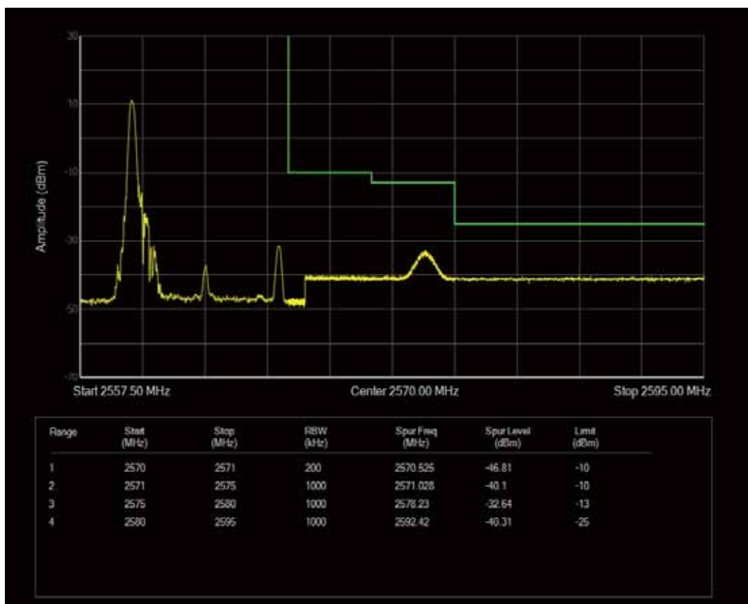
Band7 QAM16 BW=10MHz Channel=21400 RB Size=1 Position=#Max
