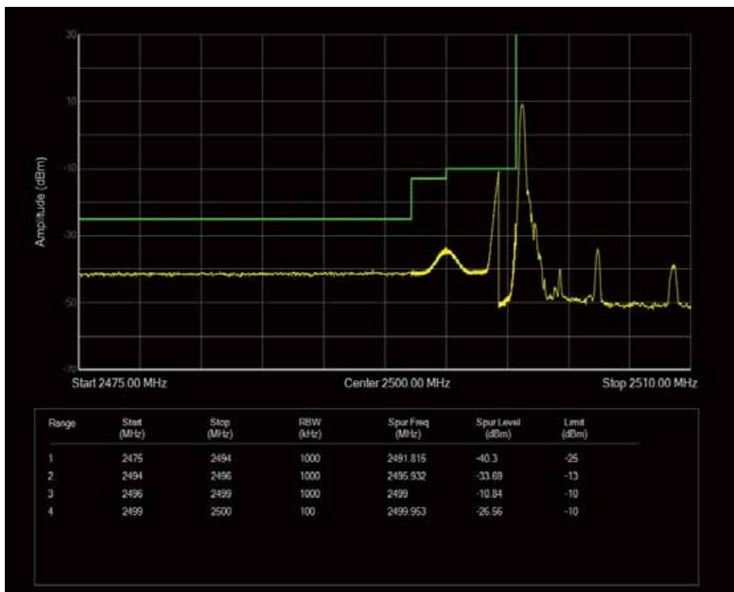
Band7 QPSK BW=5MHz Channel=20775 RB Size=25 Position=#0
