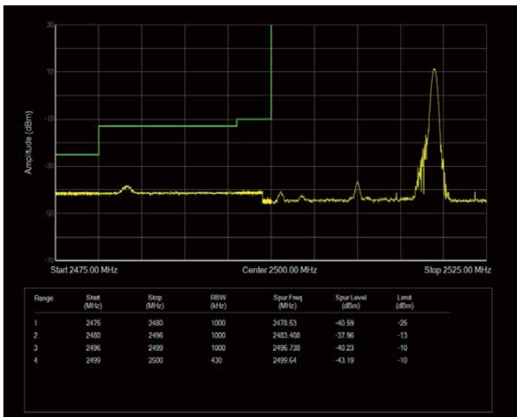
Band7 QAM16 BW=20MHz Channel=20850 RB Size=1 Position=#0
