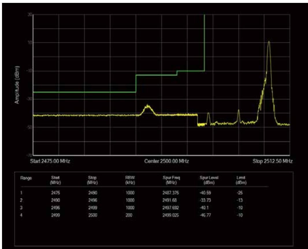
Band7 QAM16 BW=10MHz Channel=20800 RB Size=50 Position=#0
