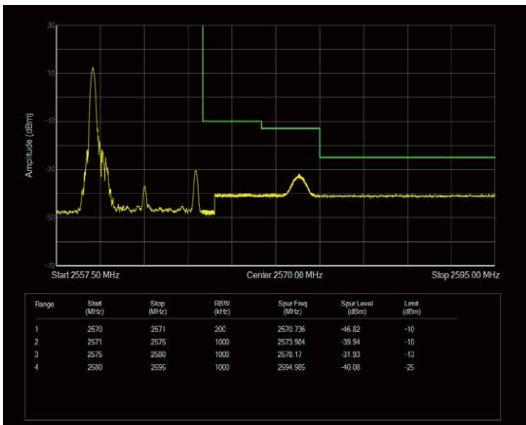
Band7 QPSK BW=10MHz Channel=21400 RB Size=50 Position=#0
