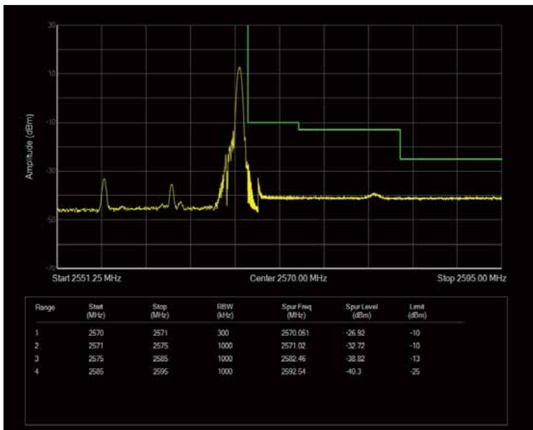
Band7 QAM16 BW=15MHz Channel=21375 RB Size=1 Position=#0
