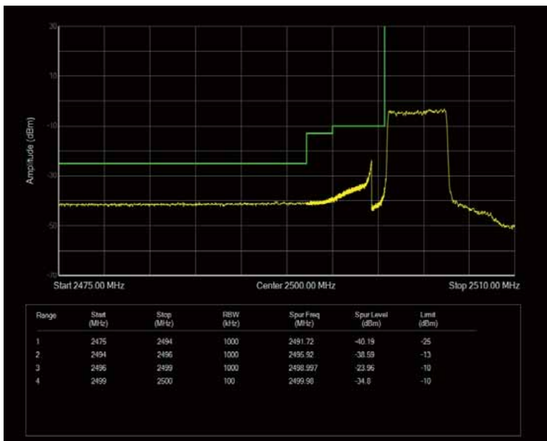
Band7 QAM16 BW=5MHz Channel=20775 RB Size=1 Position=#Max
