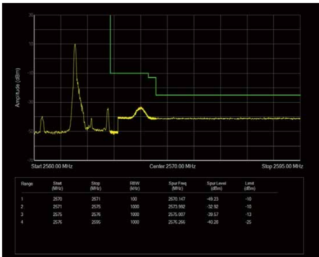
Band7 QPSK BW=5MHz Channel=21425 RB Size=25 Position=#0
