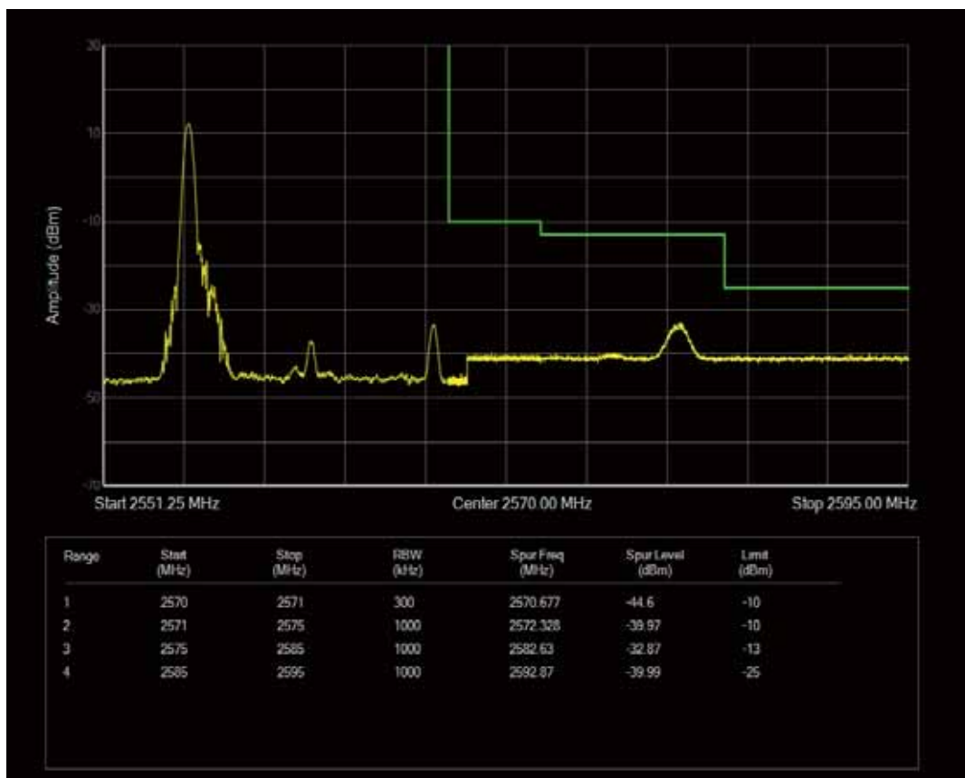
Band7 QPSK BW=15MHz Channel=21375 RB Size=75 Position=#0
