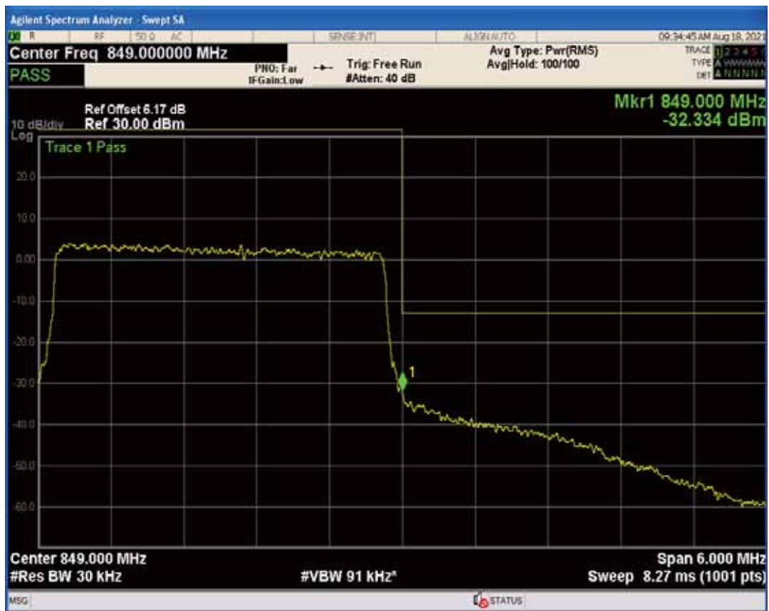
Band5 QAM16 BW=3MHz Channel=20635 RB Size=1 Position=#Max
