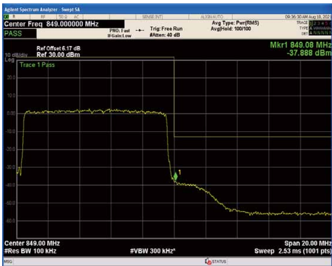
Band7 QPSK BW=5MHz Channel=20775 RB Size=1 Position=#Max
