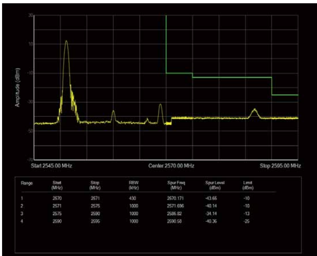
Band7 QPSK BW=20MHz Channel=21350 RB Size=100 Position=#0
