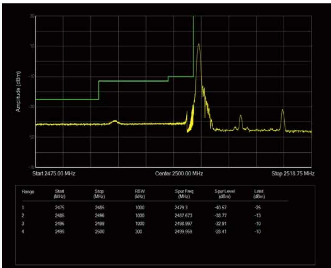
Band7 QAM16 BW=15MHz Channel=20825 RB Size=1 Position=#Max
