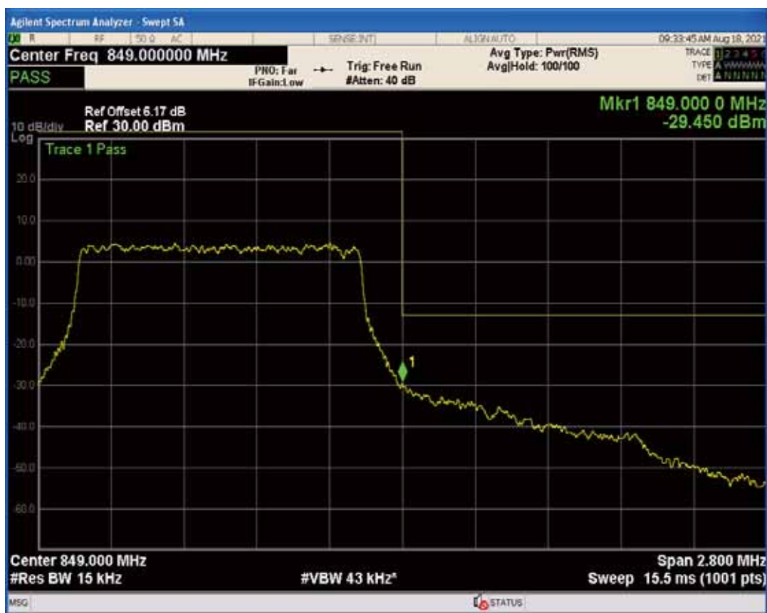
Band5 QPSK BW=1.4MHz Channel=20643 RB Size=1 Position=#Max
