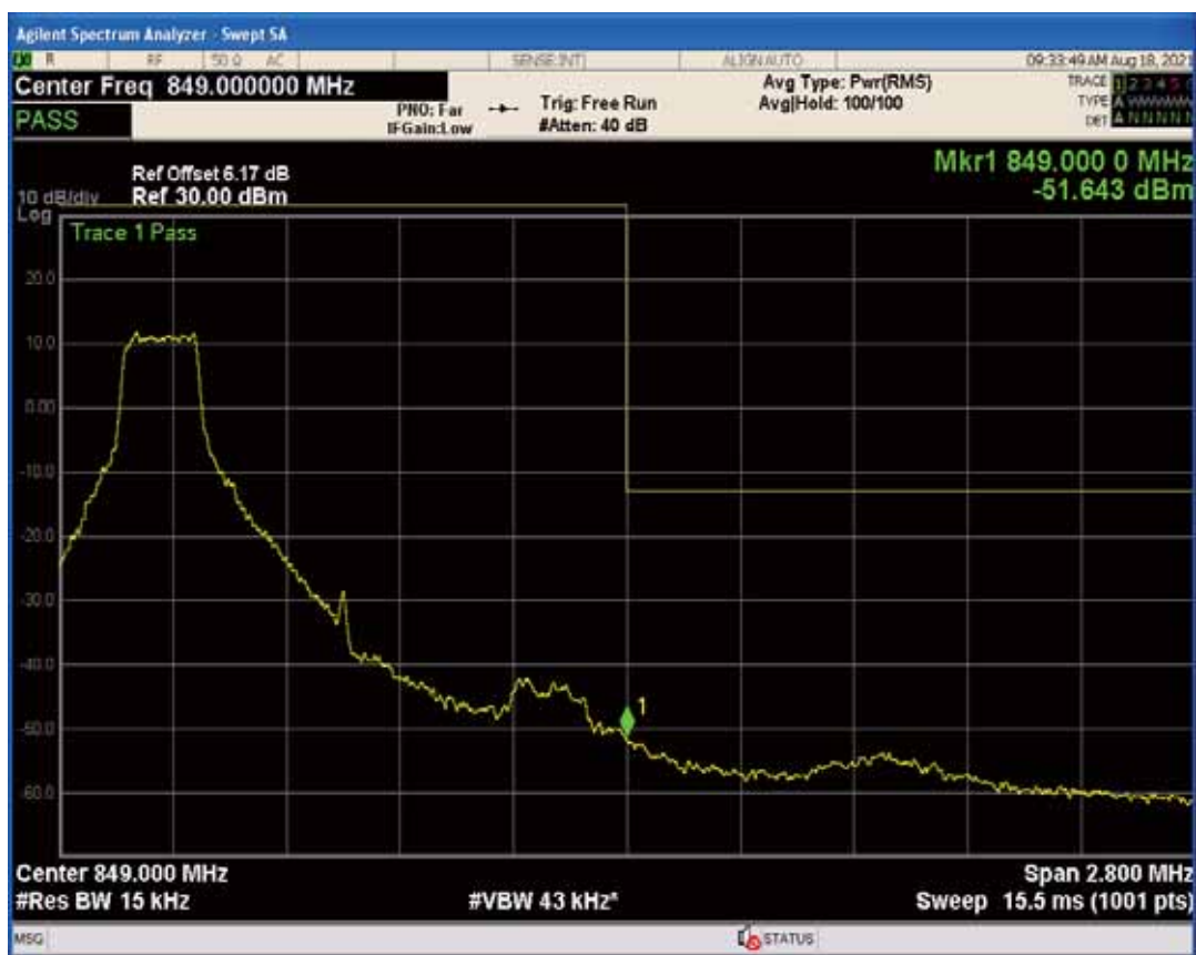
Band5 QAM16 BW=1.4MHz Channel=20643 RB Size=6 Position=#0
