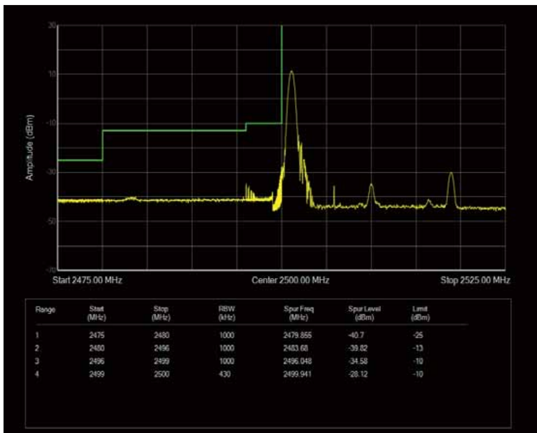
Band7 QAM16 BW=20MHz Channel=20850 RB Size=100 Position=#0
