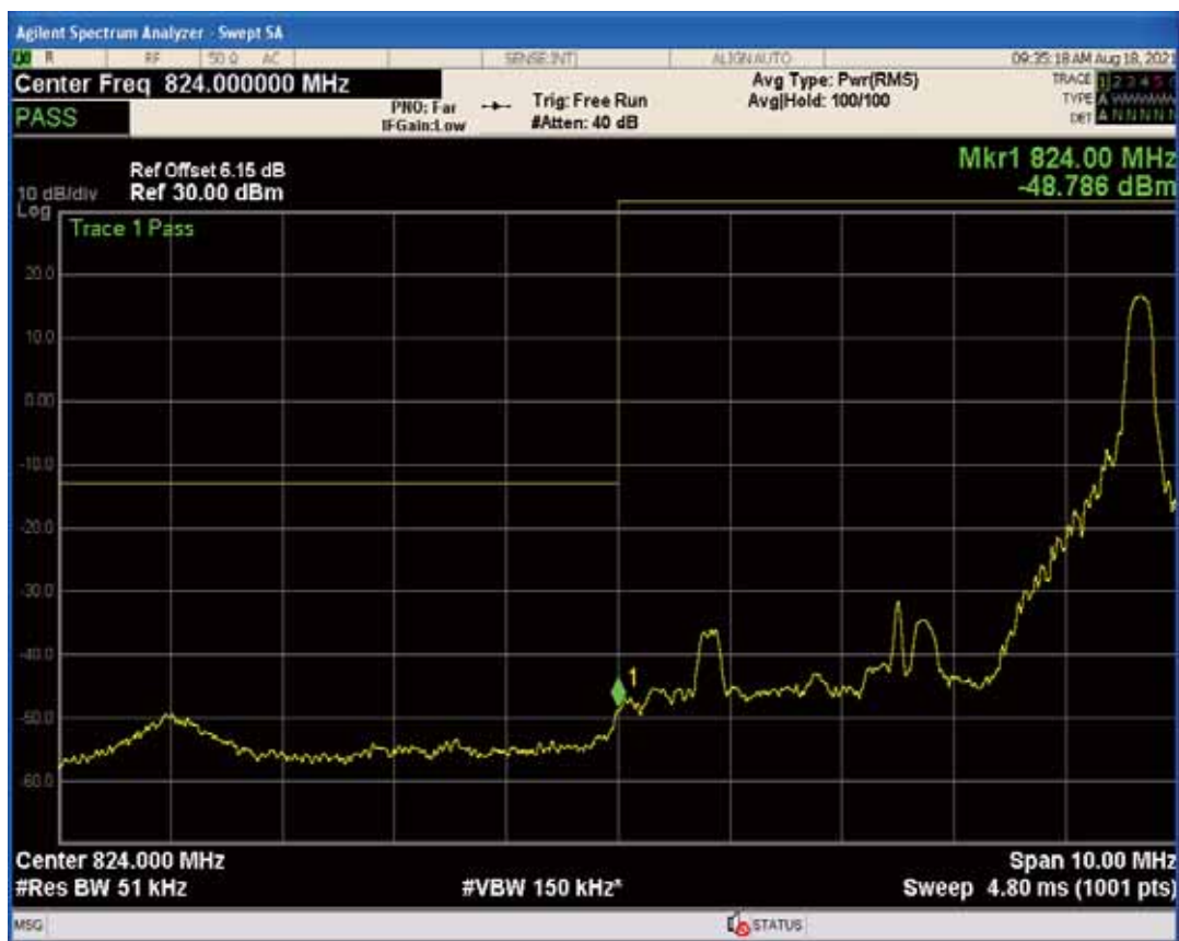
Band5 QAM16 BW=5MHz Channel=20425 RB Size=25 Position=#0
