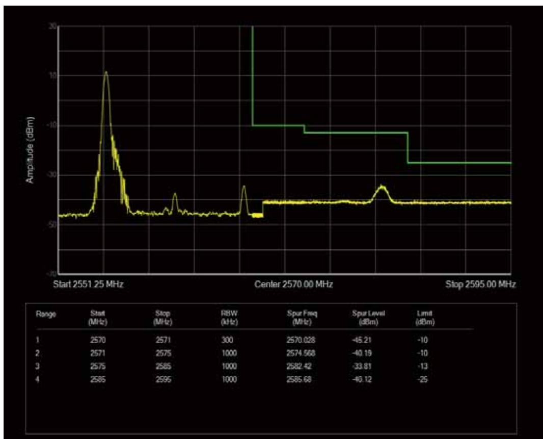
Band7 QAM16 BW=15MHz Channel=21375 RB Size=1 Position=#Max
