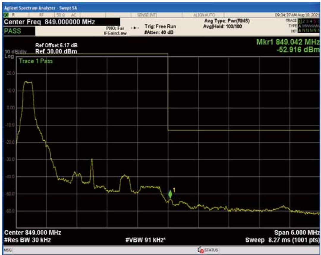
Band5 QPSK BW=3MHz Channel=20635 RB Size=15 Position=#0
