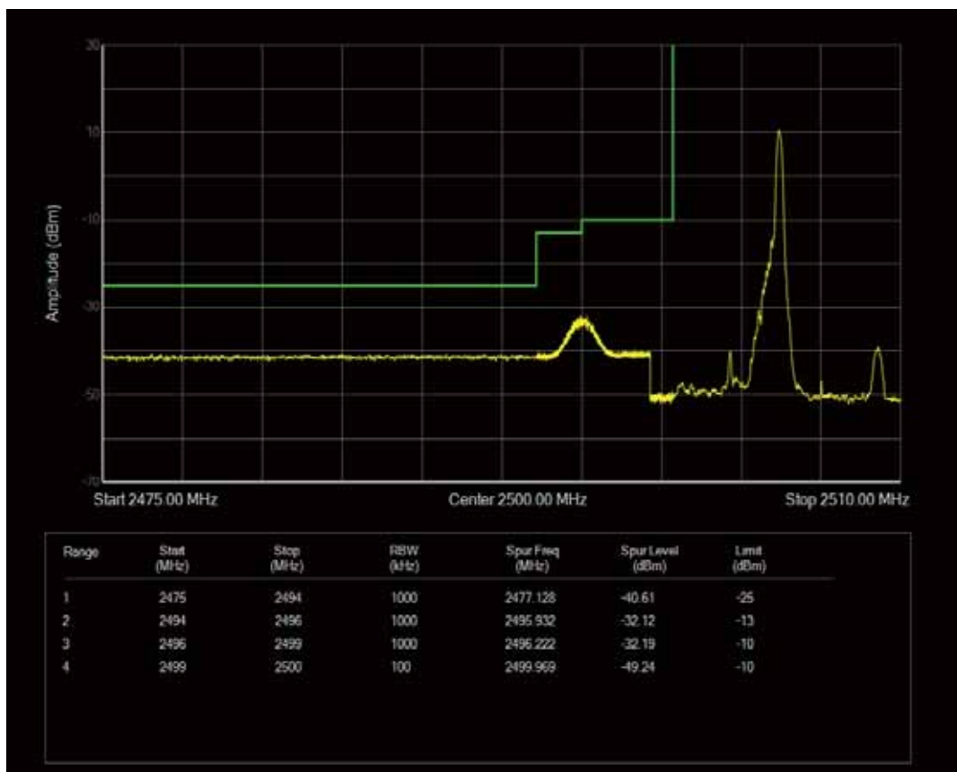
Band7 QPSK BW=5MHz Channel=20775 RB Size=1 Position=#0
