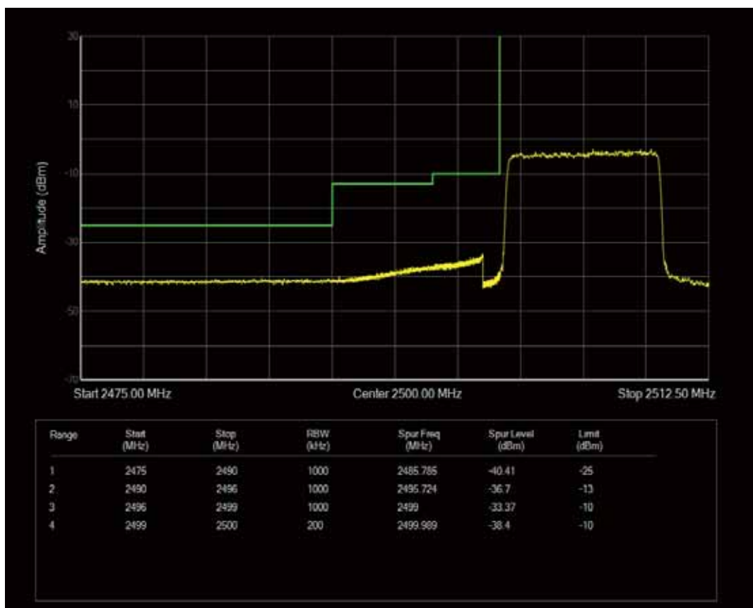
Band7 QPSK BW=10MHz Channel=20800 RB Size=1 Position=#Max
