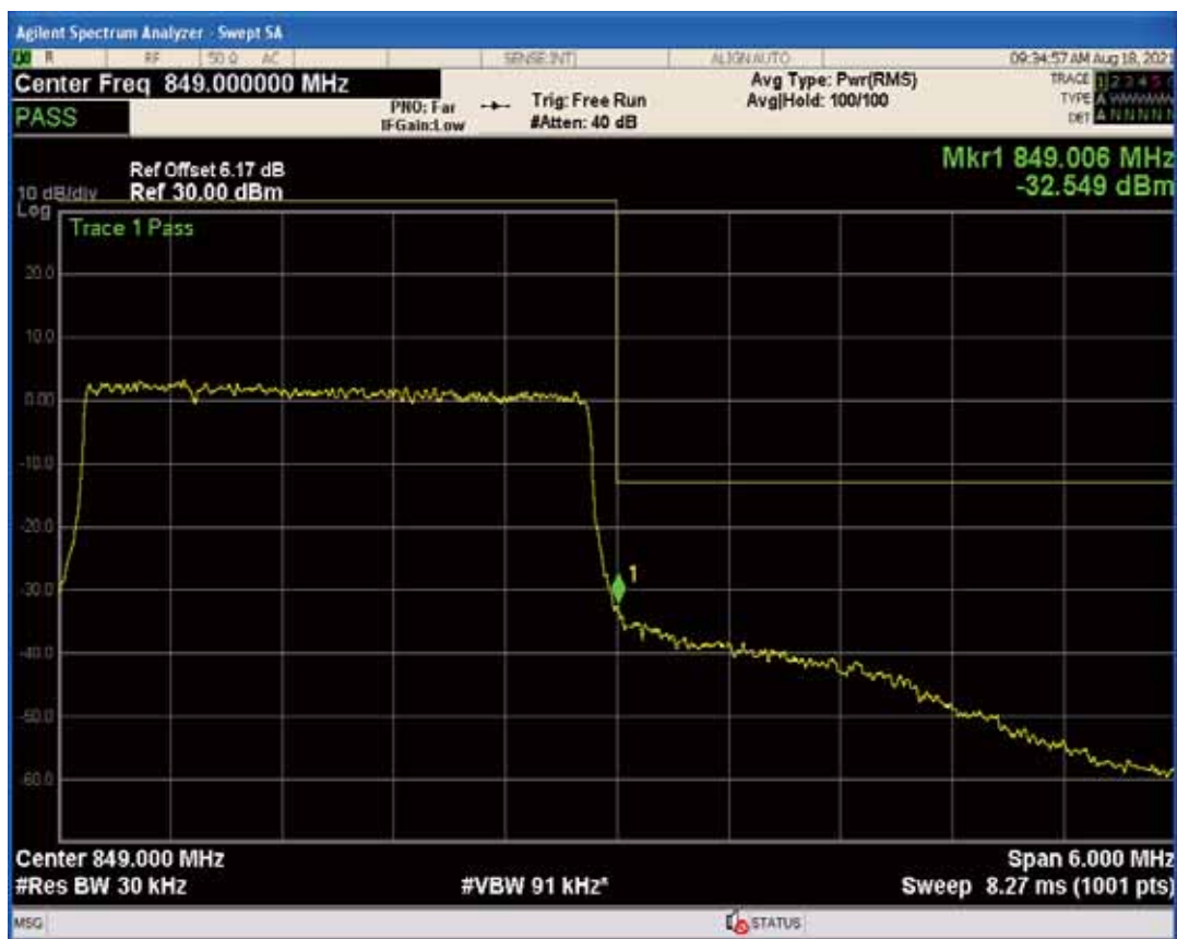
Band5 QPSK BW=5MHz Channel=20425 RB Size=1 Position=#Max
