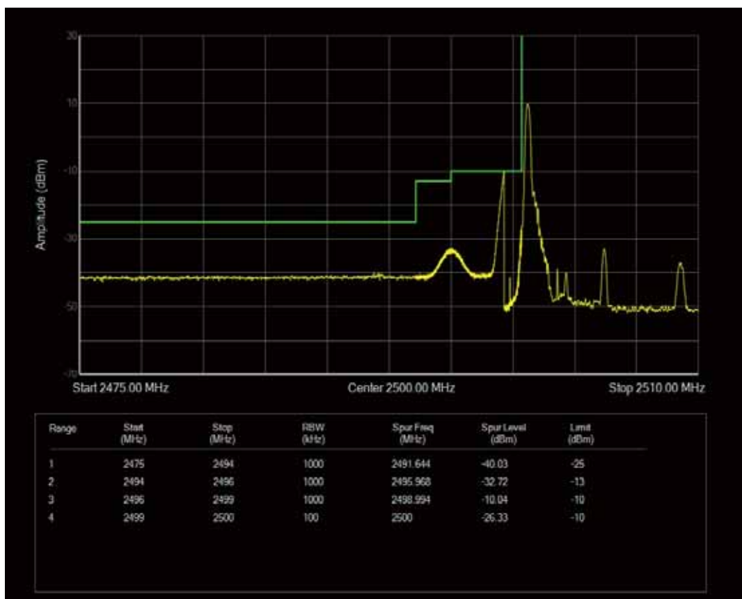
Band7 QAM16 BW=5MHz Channel=20775 RB Size=1 Position=#0
