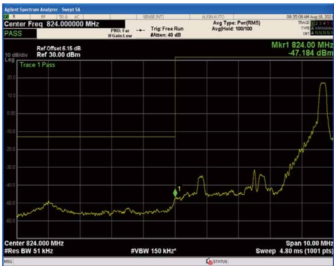
Band5 QAM16 BW=5MHz Channel=20425 RB Size=1 Position=#0
