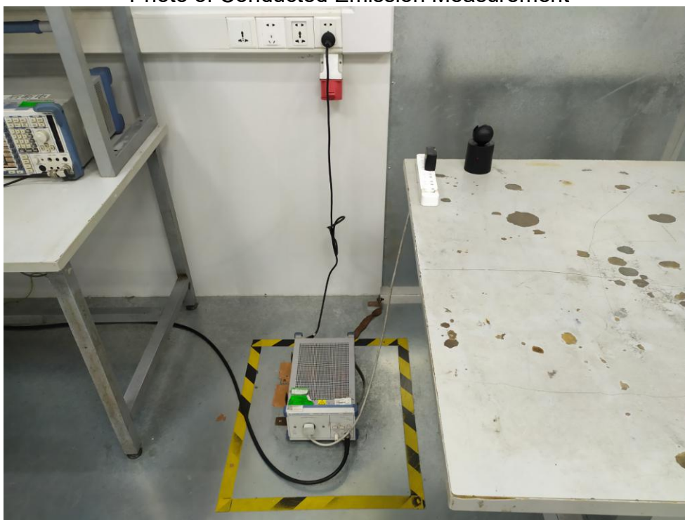
FCC ID: 2AXO2-CAPTURE360 Photo of Conducted Emission Measurement
