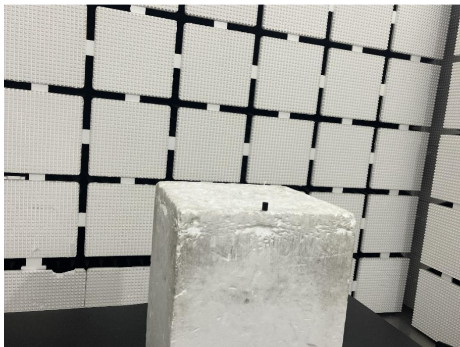
Radiation Emission Test Setup (close up)
