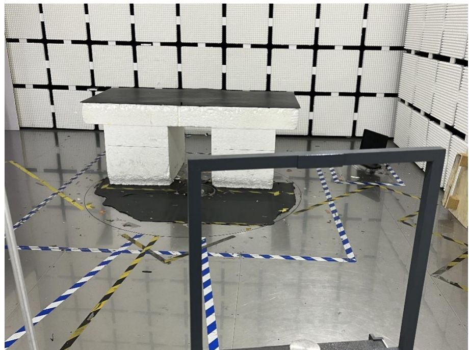
Radiation Emission Test Setup (Below 30MHz)
