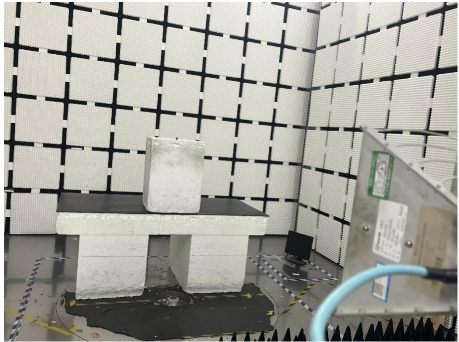
Radiation Emission Test Setup (1GHz to 18GHz)
