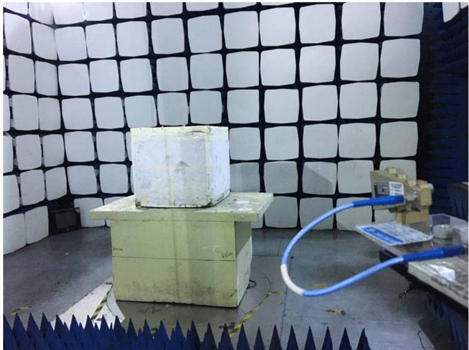
Radiation Emission Test Setup (Above 18GHz)
