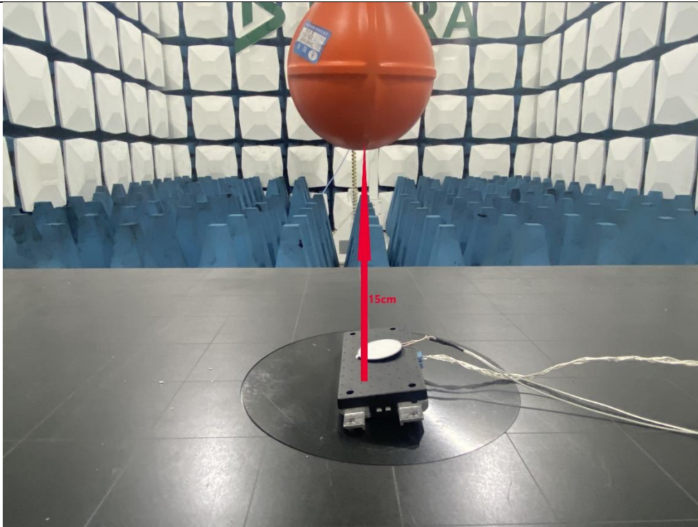
Description: RF Exposure Setup –Above 100kHz(Top)
