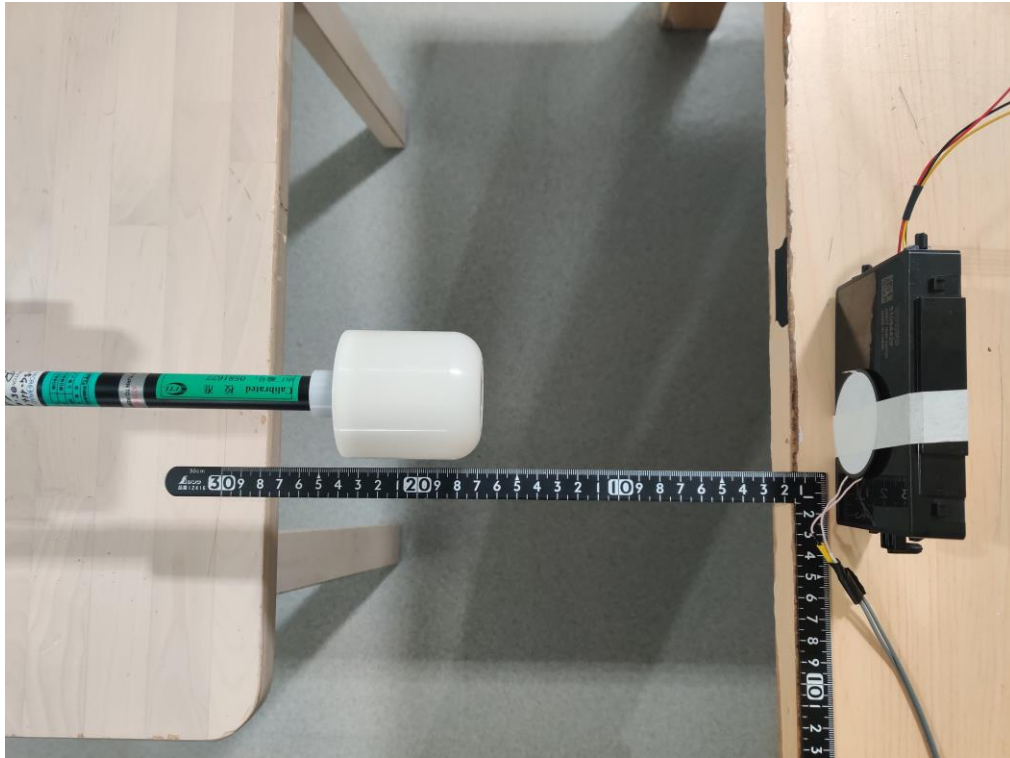
Description: RF Exposure Test Setup for Magnetic Field Emissions Test Mode 2
