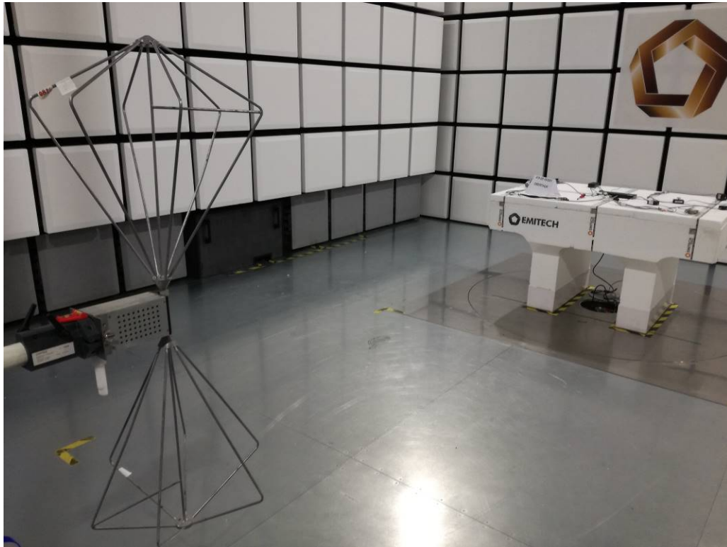
TEST SETUP PHOTO(S) – 30MHZ < FOR FREQ < 200MHZ
