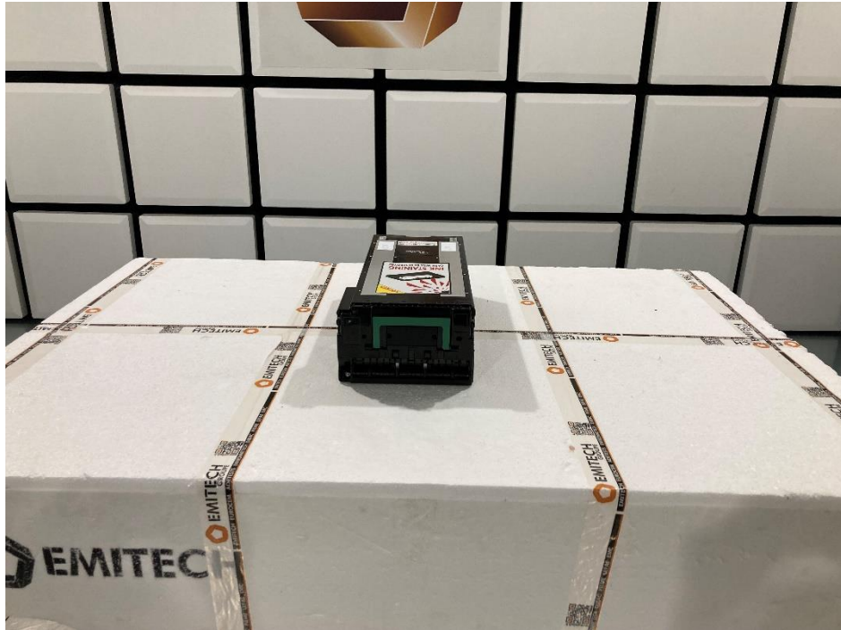
TEST SETUP PHOTO(S) - TX MODE – FOR FREQ <30MHZ
