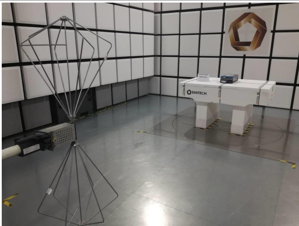
TEST SETUP PHOTO(S) – 30MHz < FOR FREQ < 200MHz
