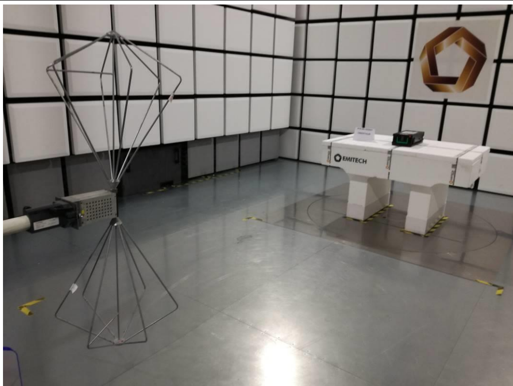
TEST SETUP PHOTO(S) – 30MHz < FOR FREQ < 200MHz
