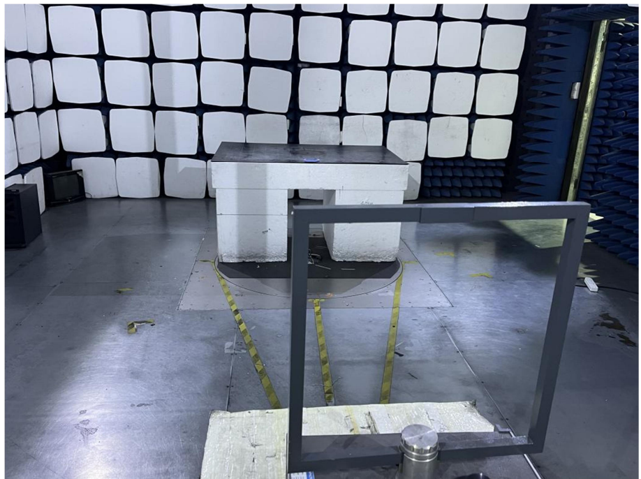
Radiation Emission Test Setup (Below 30MHz)
