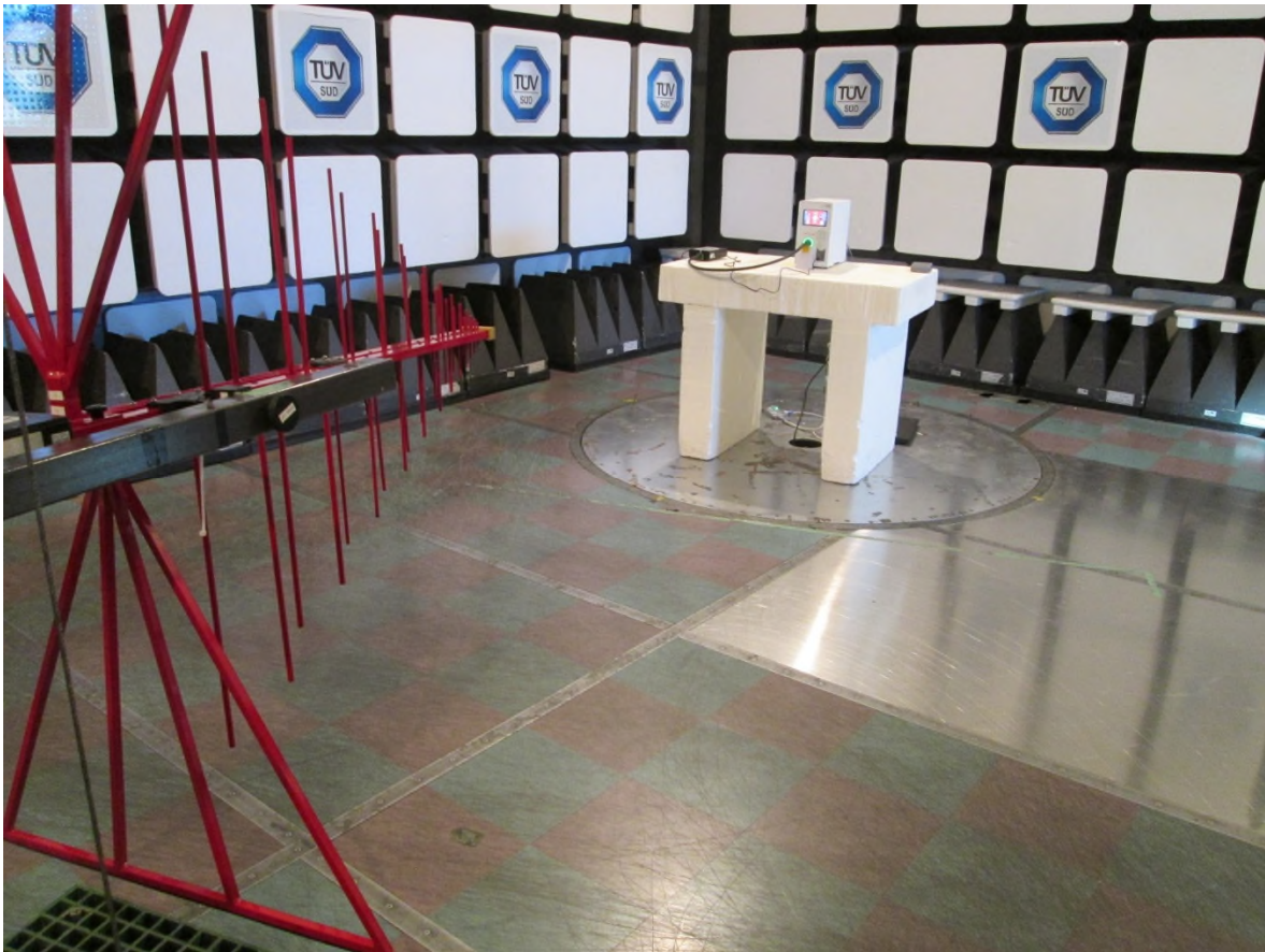
Test setup photo 2 Radiated measurements, 30 MHz – 1 GHz
