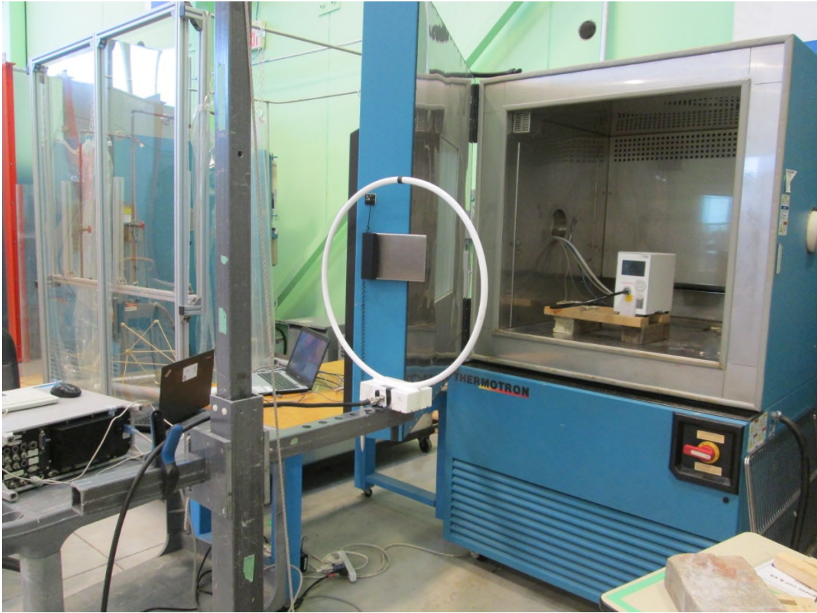
Test setup photo 5 Frequency Stability at Extreme Temperatures
