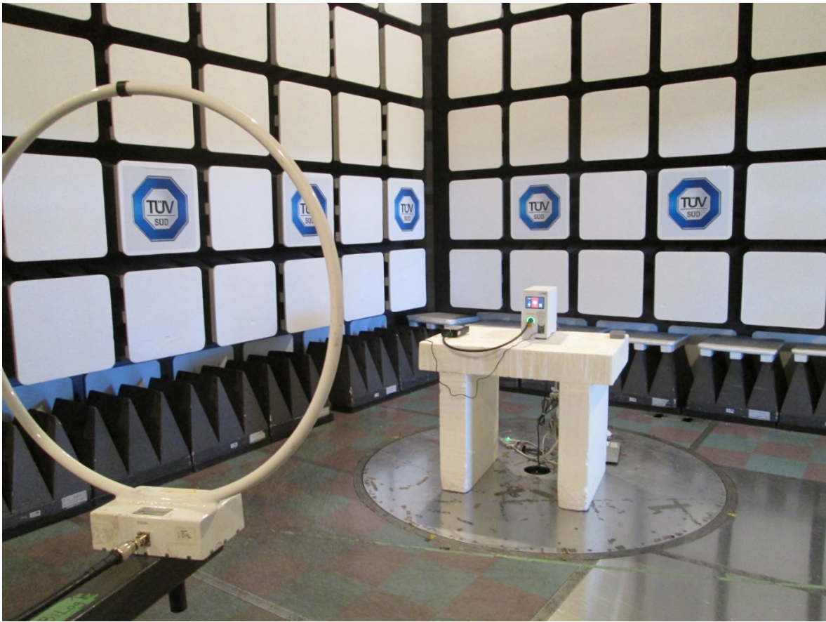
Test setup photo 1 Radiated measurements, 9 kHz – 30 MHz
