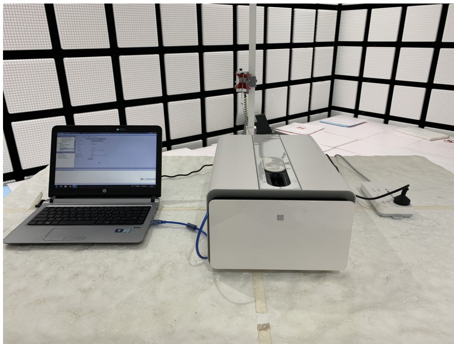
Radiated spurious emission Test Setup-2(Above 1GHz)
