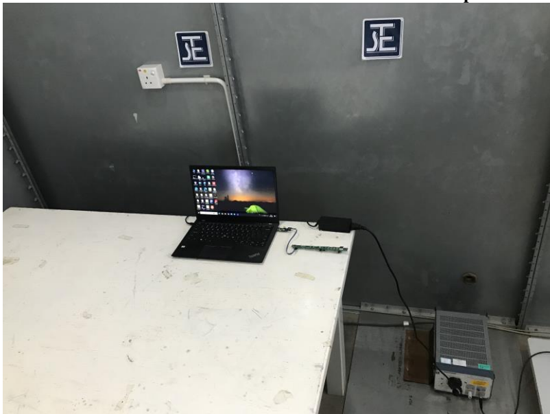
Measurement of Conducted Emission Test Set Up
