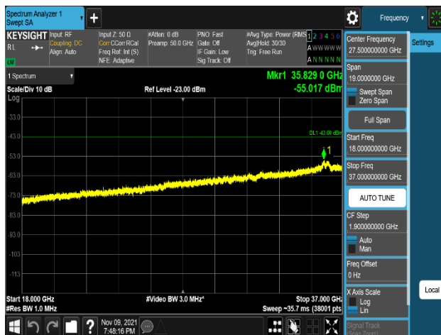
Plot 8-46. Conducted Spurious Emission Plot 18 GHz to 37 GHz (LTE_B48_10M_16QAM - Low Channel, Port 0)
