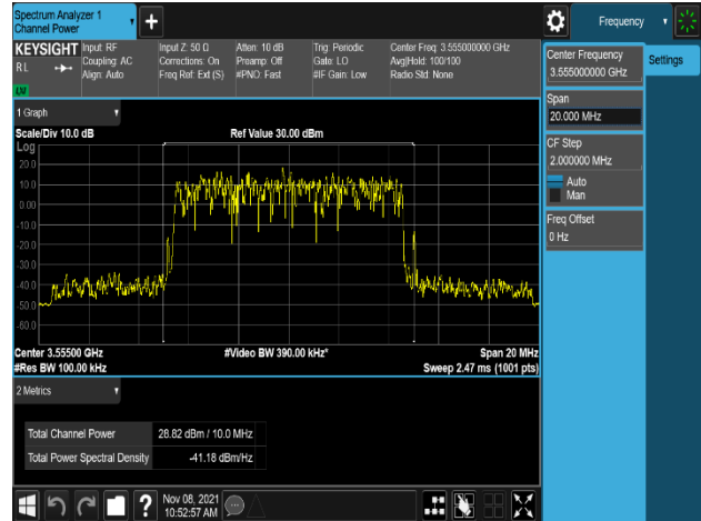
Plot 8-23. Equivalent Isotropic Radiated Power Plot (LTE_B48_10M_QPSK - Low Channel, Port 1)
