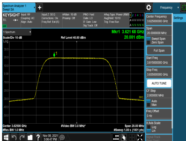
Plot 8-14. Power Spectral Density Plot (LTE_B48_10M_64QAM - Mid Channel, Port 0)
