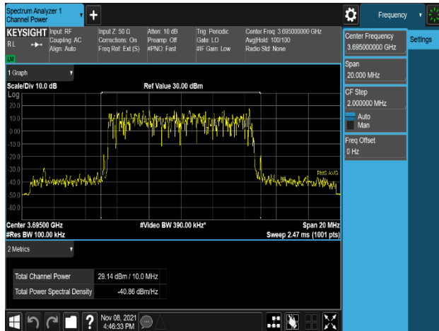
Plot 8-24. Equivalent Isotropic Radiated Power Plot (LTE_B48_10M_16QAM - High Channel, Port 0)
