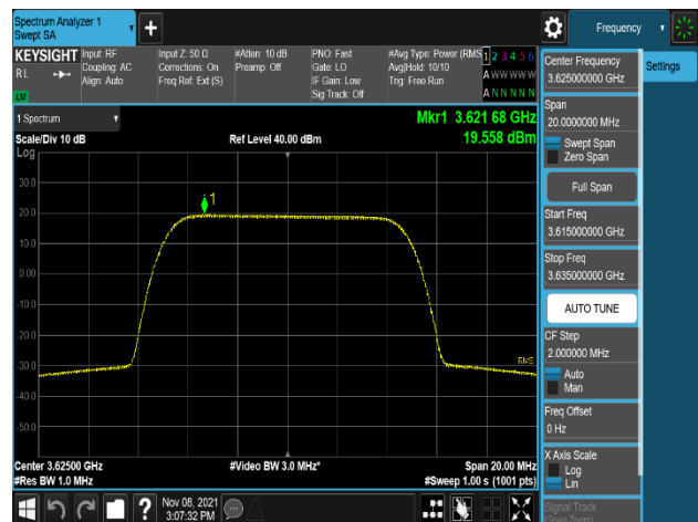
Plot 8-15. Power Spectral Density Plot (LTE_B48_10M_64QAM - Mid Channel, Port 1)
