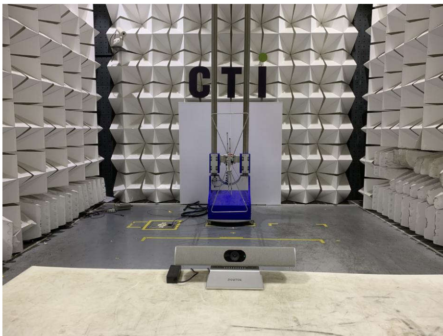
Radiated spurious emission Test Setup-1(Below 1GHz)
