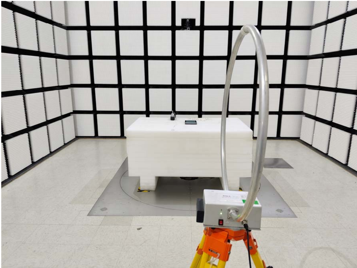
Radiated Emission 9 kHz-30 MHz Ground-parallel View
