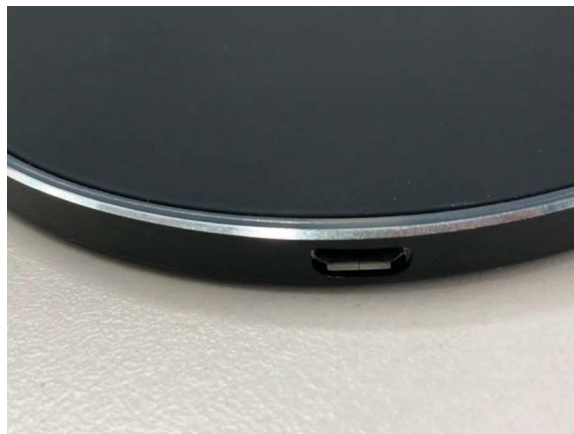
Fig 3. Micro-B Power input port
