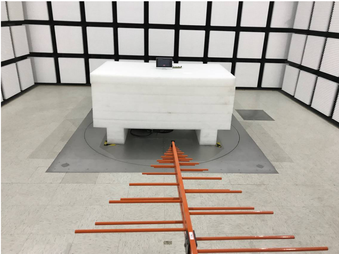
Radiated Emission Below 1GHz View- PoE power Supply mode
