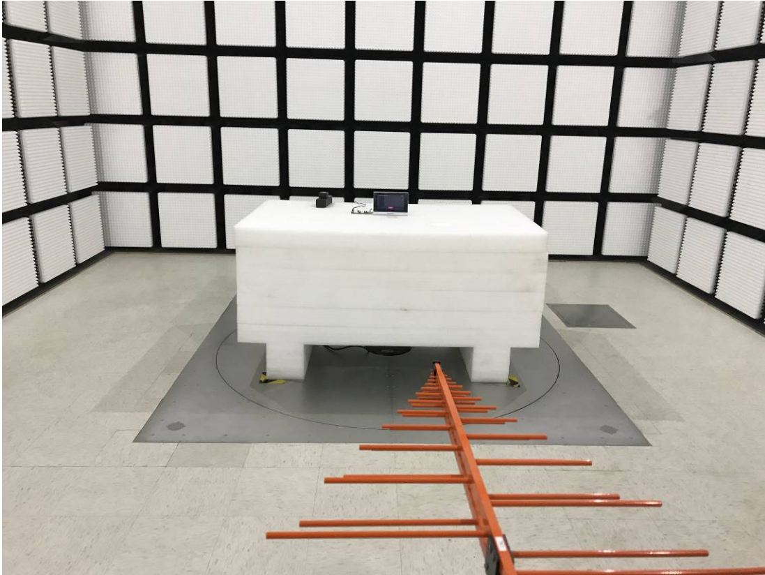
Radiated Emission Below 1GHz View- PoE power Supply mode
