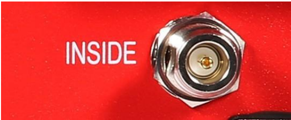
A1 — N-type Female for INSIDE cable and antenna
