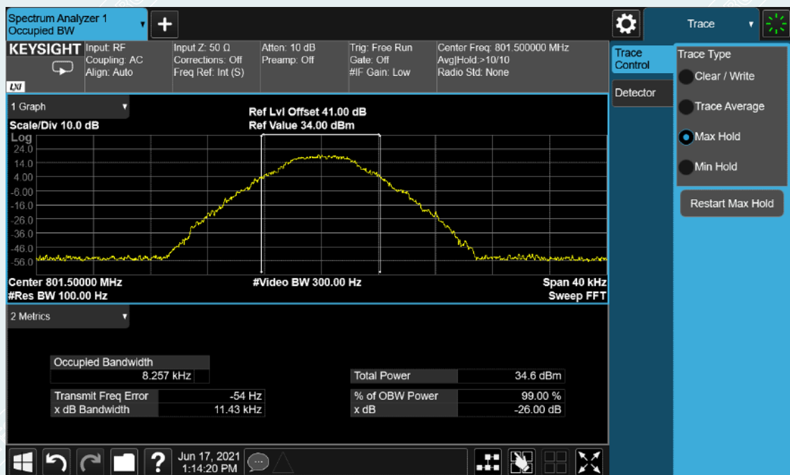
Middle Frequency: 801.5MHz, Output occupied BW (with the input signal amplitude set 3 dB above the AGC threshold)
