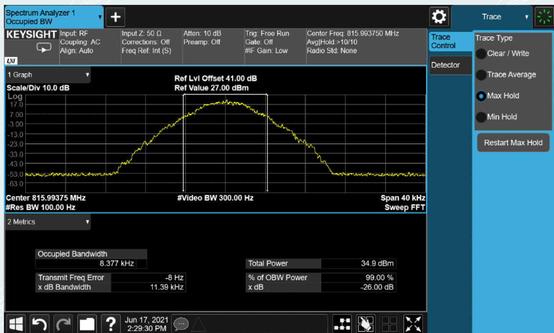
High Frequency: 815.99375MHz, Output occupied BW (with the input signal amplitude set 3 dB above the AGC threshold)
