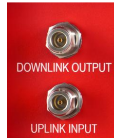
A3, A4 — N-type Female for INSIDE cable and Serving antenna
