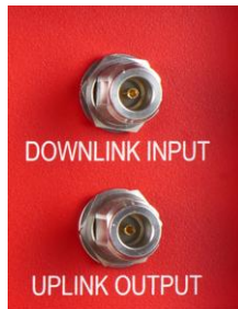
A1, A2— N-type Female for OUTSIDE cable and donor antenna
