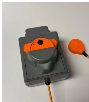
Figure 3 – FD-100 Sensor Unit placed in the Wall Unit attached with Floor Unit and powered by an external battery pack
