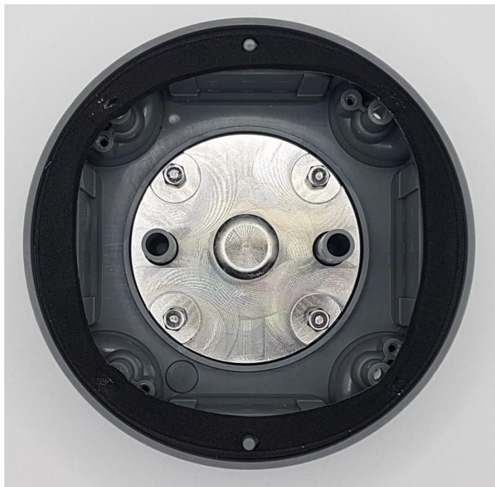
TP-400R8 Bottom Assembly with Circuit Cards Removed
