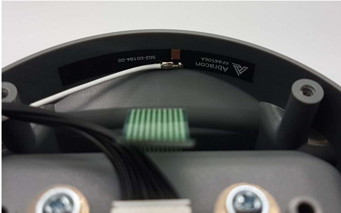
TP-400V Antenna Placement View
