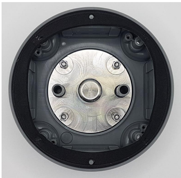
TP-400V Bottom Assembly with Circuit Cards Removed
