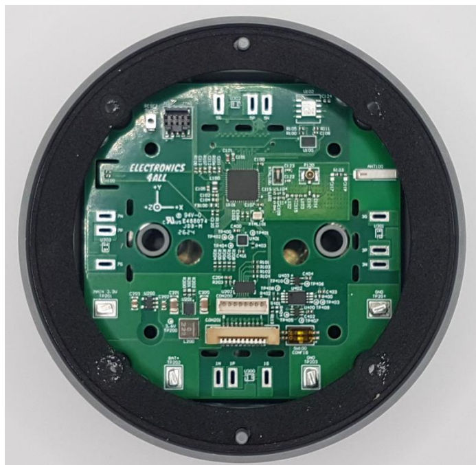
TP-400V Bottom Assembly with Circuit Cards Installed
