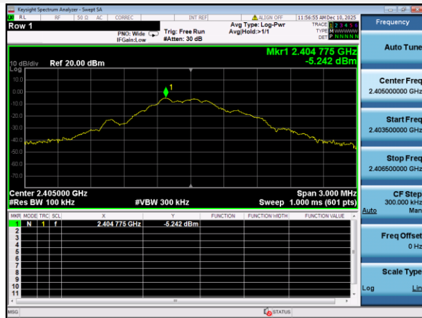
GFSK (1Mbps) LOW CHANNEL, CARRIER LEVEL
