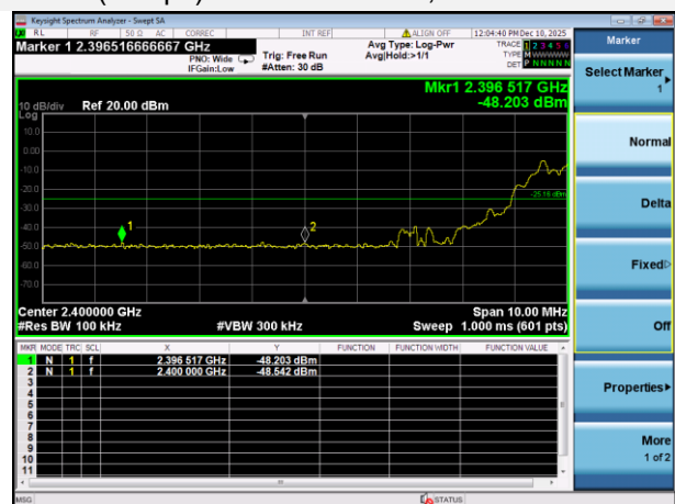
GFSK (2Mbps) LOW CHANNEL, BAND EDGE
