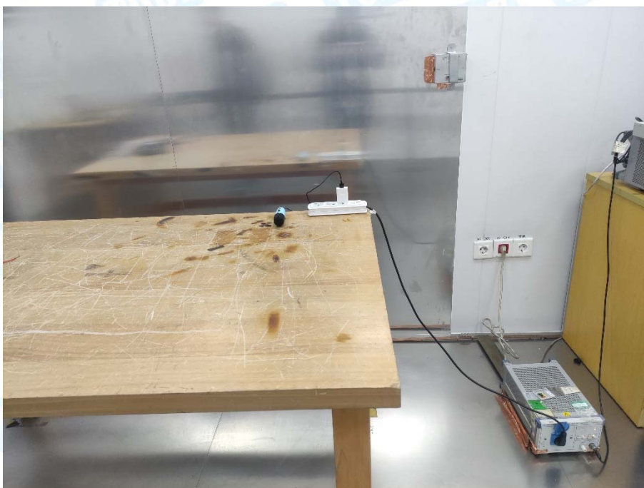
Photo of Setup for Conducted Emission
