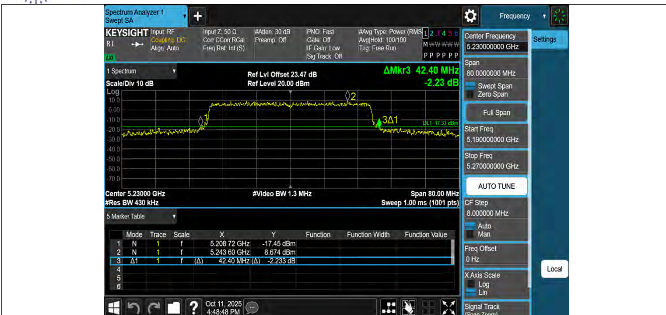
The screenshot displays a Keysight Spectrum Analyzer interface. The main display shows a spectrum plot with a yellow signal trace. A green horizontal line indicates the reference level at 20.00 dBm. A marker labeled '2' is placed on the signal trace at 5.22120 GHz with a level of 8.265 dBm. Another marker labeled '3Δ1' is placed on the signal trace at 5.20928 GHz with a level of -17.86 dBm. The center frequency is 5.23000 GHz, and the span is 80.00 MHz. The resolution bandwidth (RBW) is 430 kHz, and the video bandwidth (VBW) is 1.3 MHz. The sweep rate is 1.00 ms (1001 pts). The interface includes various control panels for input, attenuation, and measurement settings, as well as a settings panel on the right for center frequency, span, and sweep parameters. Keysight Spectrum Analyzer 1 Swept SA KEYSIGHT Input RF Coupling 10C Align Auto Input Z 50 Ω Corr C Corr R Cal Freq Ref Int (S) #Atten 30 dB PNO Fast Gate Off IF Gain Low Sig Track Off #Avg Type Power (RMS) Avg/Hold 100/100 Trig Free Run M www www p p p p p 1 Spectrum Scale/Div 10 dB Log Ref Lvl Offset 23.39 dB Ref Level 20.00 dBm ΔMkr3 40.80 MHz 0.02 dB 3Δ1 0.11 -17.74 dBm Center 5.23000 GHz #Res BW 430 kHz #Video BW 1.3 MHz Span 80.00 MHz Sweep 1.00 ms (1001 pts) 5 Marker Table Mode Trace Scale X Y Function Function Width Function Value 1 N 1 f 5.209 28 GHz -17.86 dBm 2 N 1 f 5.221 20 GHz 8.265 dBm 3 Δ1 1 f (Δ) 40.80 MHz (Δ) 0.02277 dB 4 5 6 Center Frequency 5.230000000 GHz Span 80.00000000 MHz Swept Span Zero Span Full Span Start Freq 5.190000000 GHz Stop Freq 5.270000000 GHz AUTO TUNE CF Step 8.0000000 MHz Auto Man Freq Offset 0 Hz X Axis Scale Log Lin Signal Trace (Sweep, Trace)
