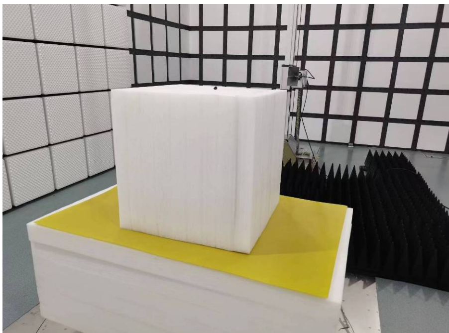
Photo of Radiated Emission Measurement (Above 1G)
