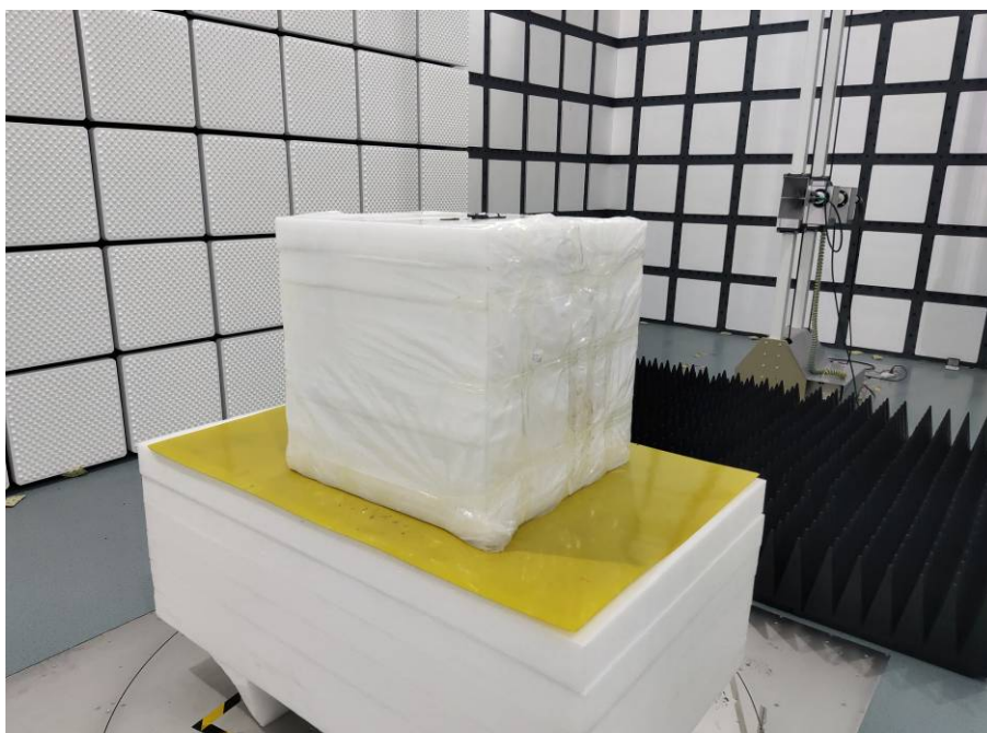
Photo of Radiated Emission Measurement (Above 1G)
