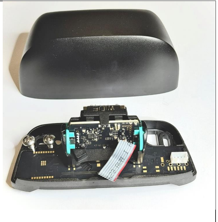
Fig. 5. Racon-D-NA (Bottom View) (a) Radar Cover with LED Window (b) Radar fully assembled
