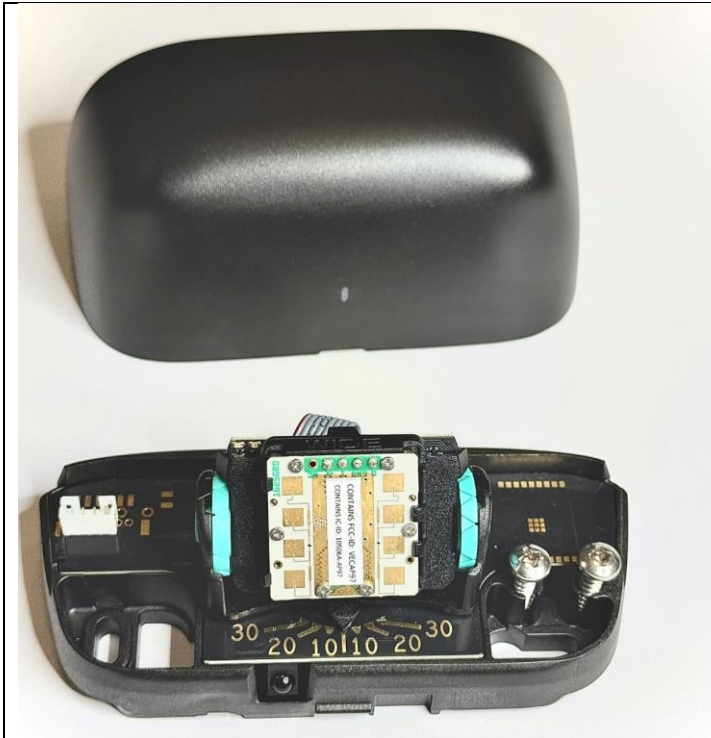
Fig. 4. Racon-D-NA (Top View) (a) Radar Cover with LED Window (b) Radar fully assembled
