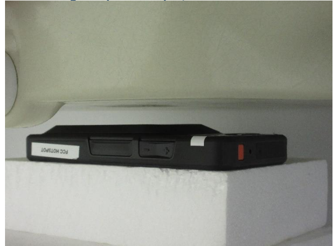
Testing Setup for Hotspot, Rear Face at 10 mm
