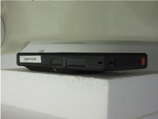
Testing Setup for Hotspot, Front Face at 10 mm
