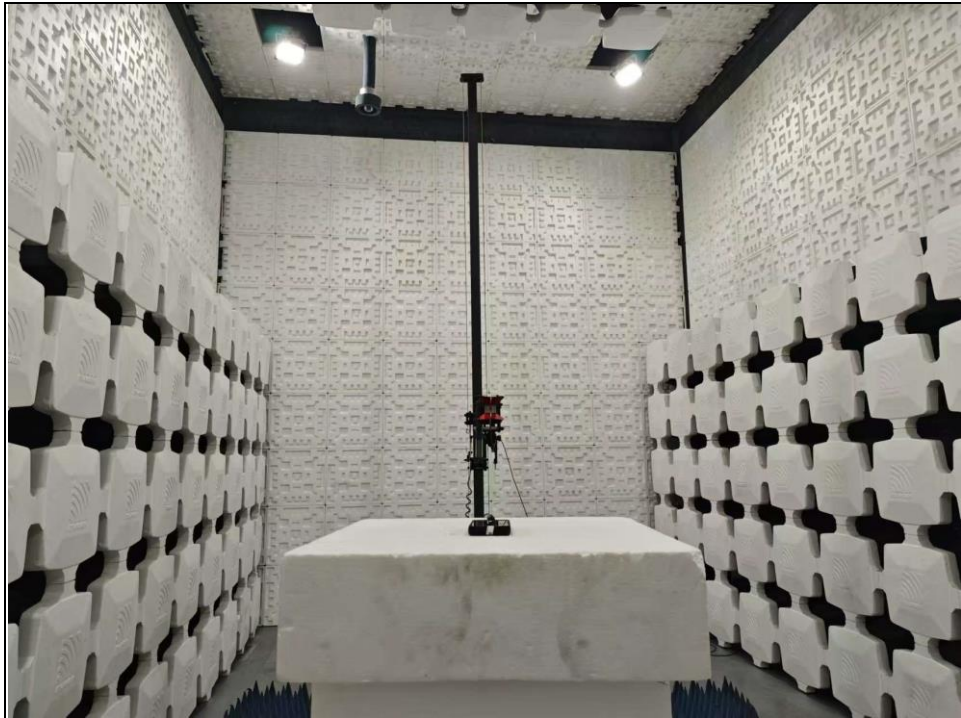
Radiated emission test: Frequency Range < Above 1GHz >
