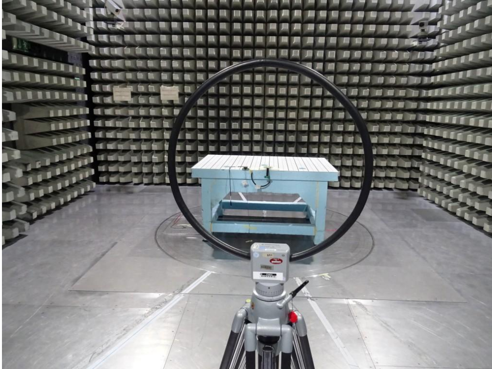
Photo 1 Radiated Test Setup from 9 kHz to 30 MHz
