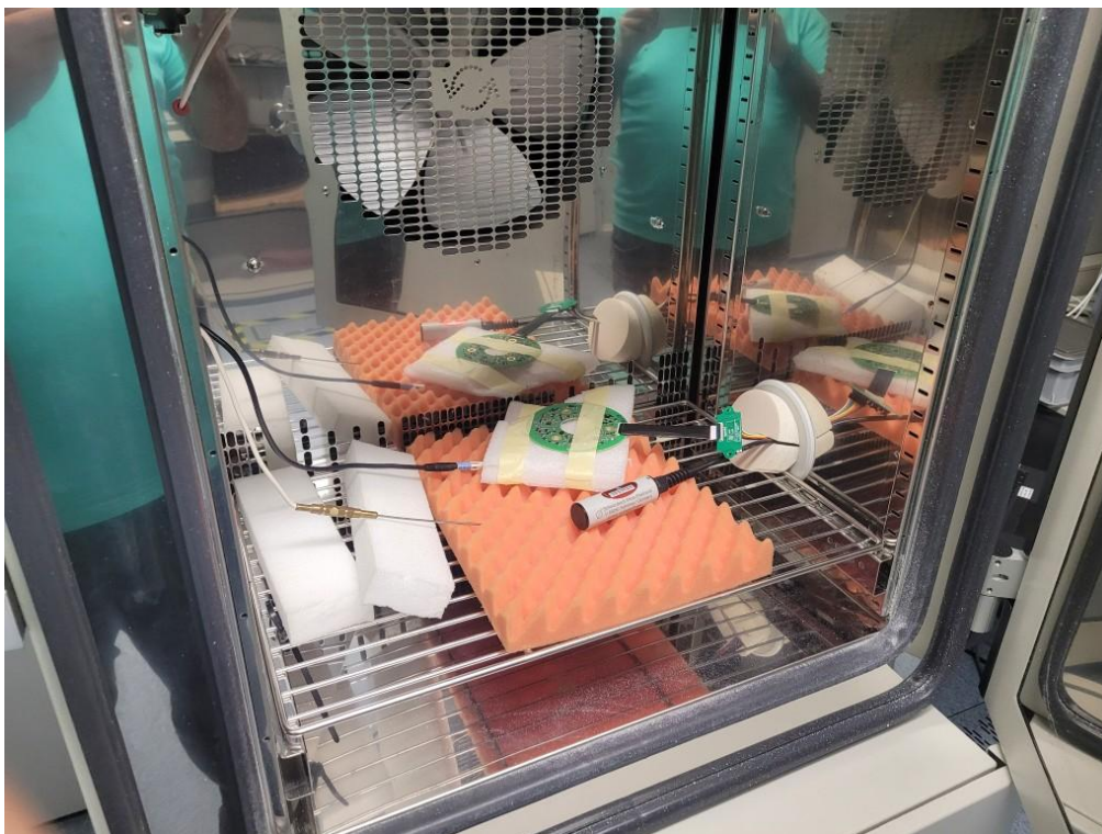
Photo 5 Bench test set up for (99% / 20 dB Bandwidth and Frequency Stability) (@ Ambient + Extreme Temperature, as required)
