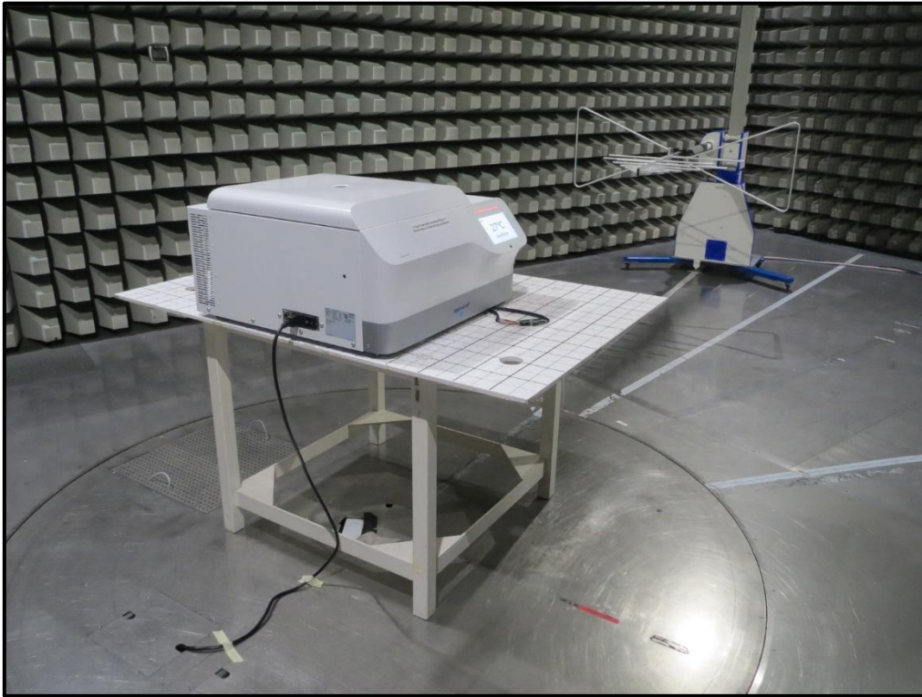
Photo 3 Radiated Test Setup from 30 MHz to 1 GHz
