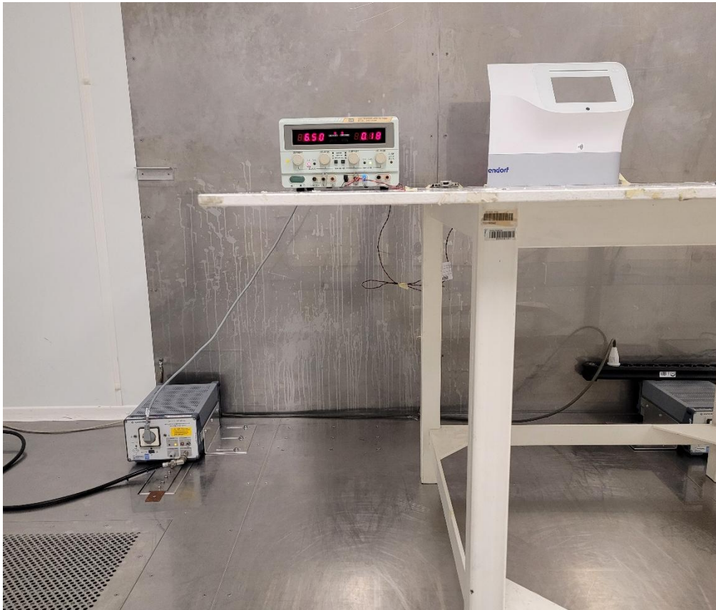
Photo 6 AC conducted emission
