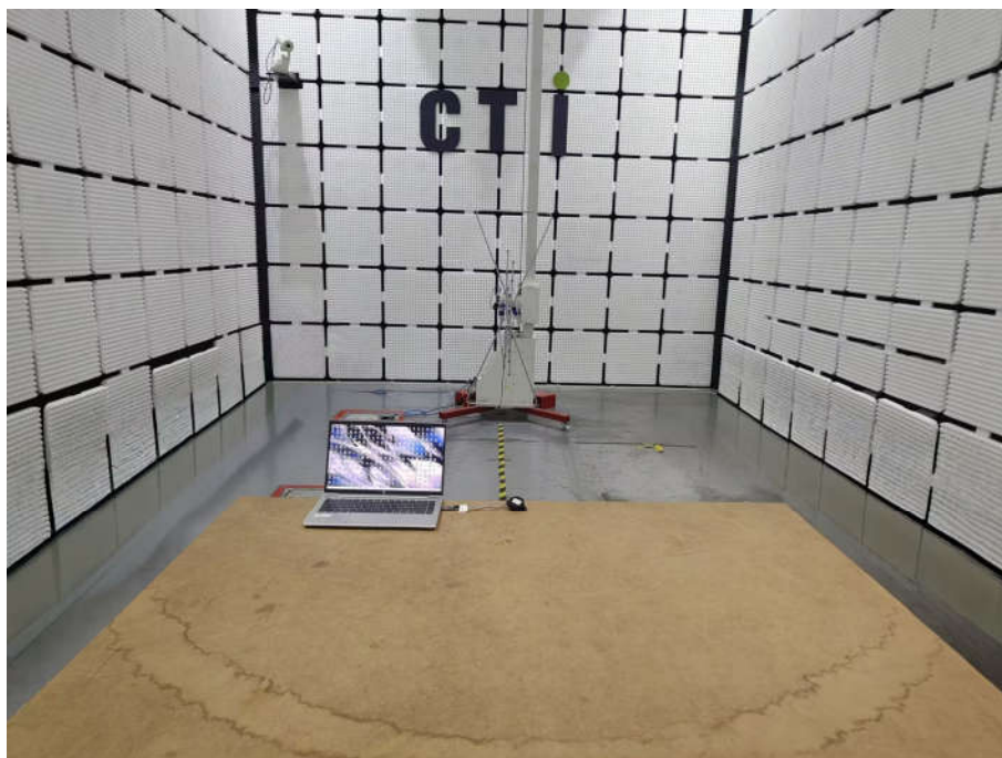
Radiated spurious emission Test Setup-1(Below 1GHz)
