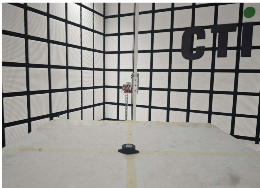
Radiated spurious emission Test Setup-2(Above 1GHz)
