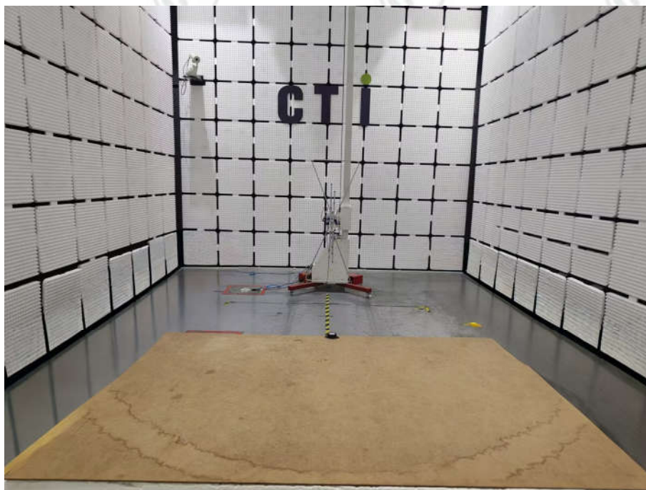
Radiated spurious emission Test Setup-1(Below 1GHz)
