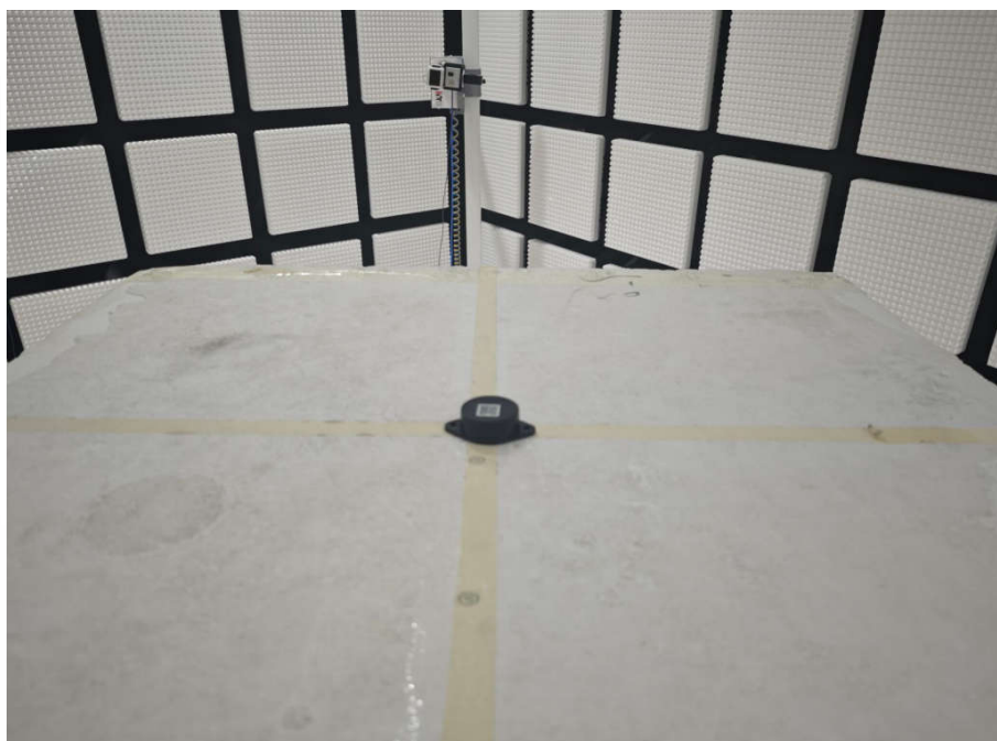
Radiated spurious emission Test Setup-3(Above 18GHz)
