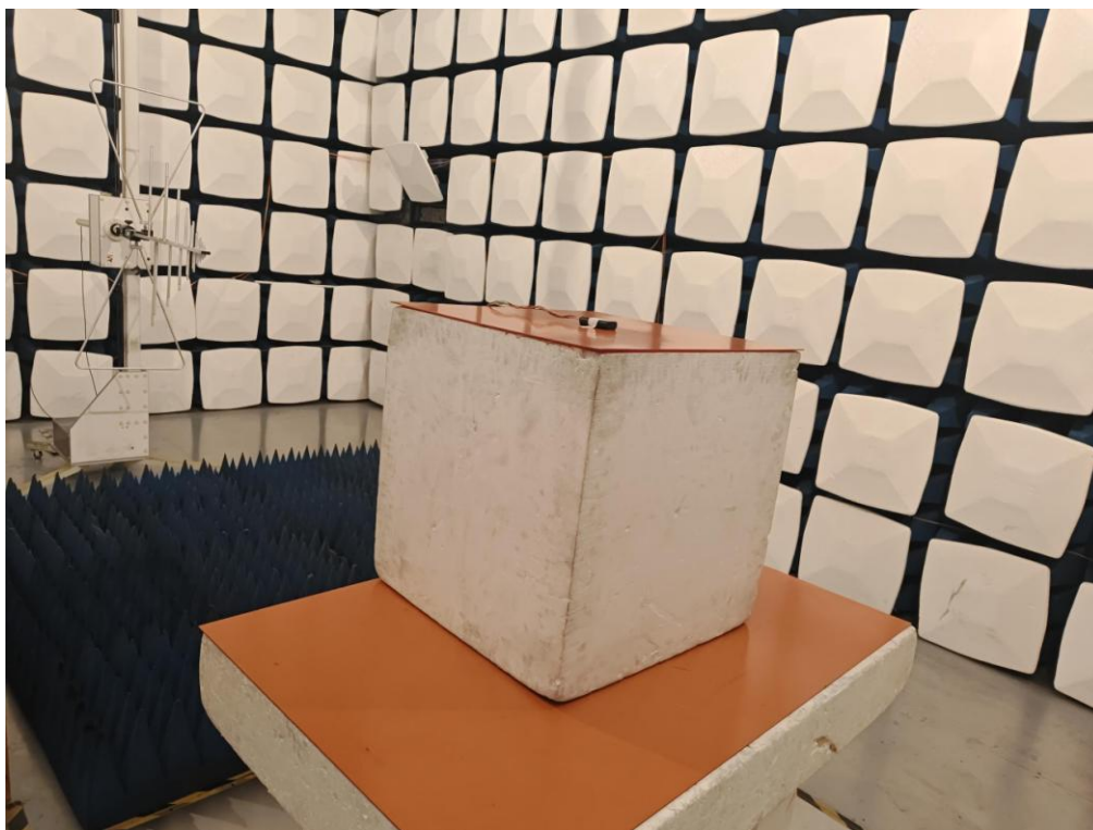
Radiated Emissions Measurement (Below 1GHz)
