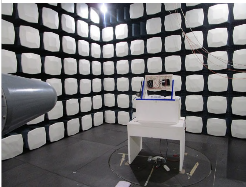
Photograph 4: EUT test setup in the fully anechoic chamber, overview
