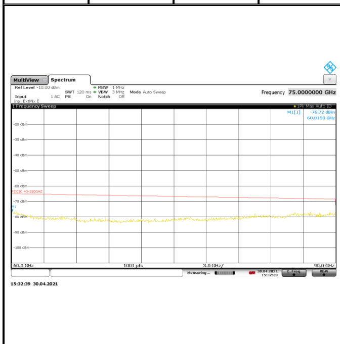
Plot# 60 Radiated Emission 60-90GHz
